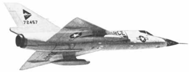
F-106. Now operational with the Air Defense Command of the United States Air Force. A later, faster sister to the F-102. In 1959, it was clocked at 1,525.95 miles per hour—or 2.3 times the speed of sound.
