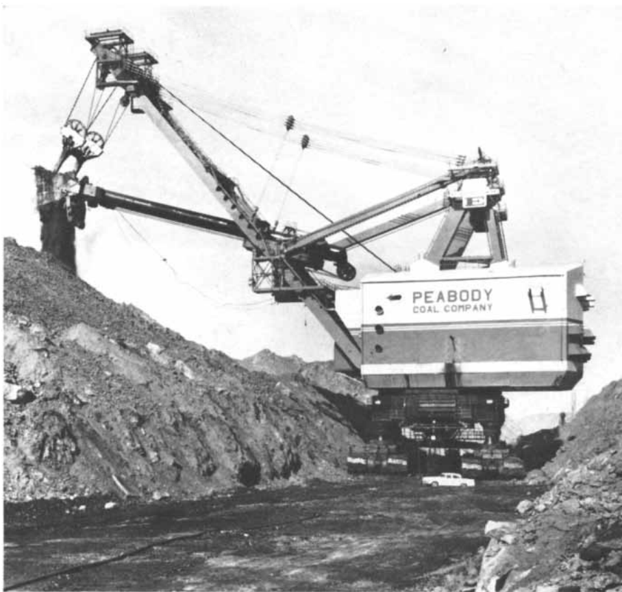
GIANT POWER SHOVEL is used for strip-mining in a coal mine near St. Louis. The bucket can move 250 tons of earth in one bite. Automobile indicates size of machine.
