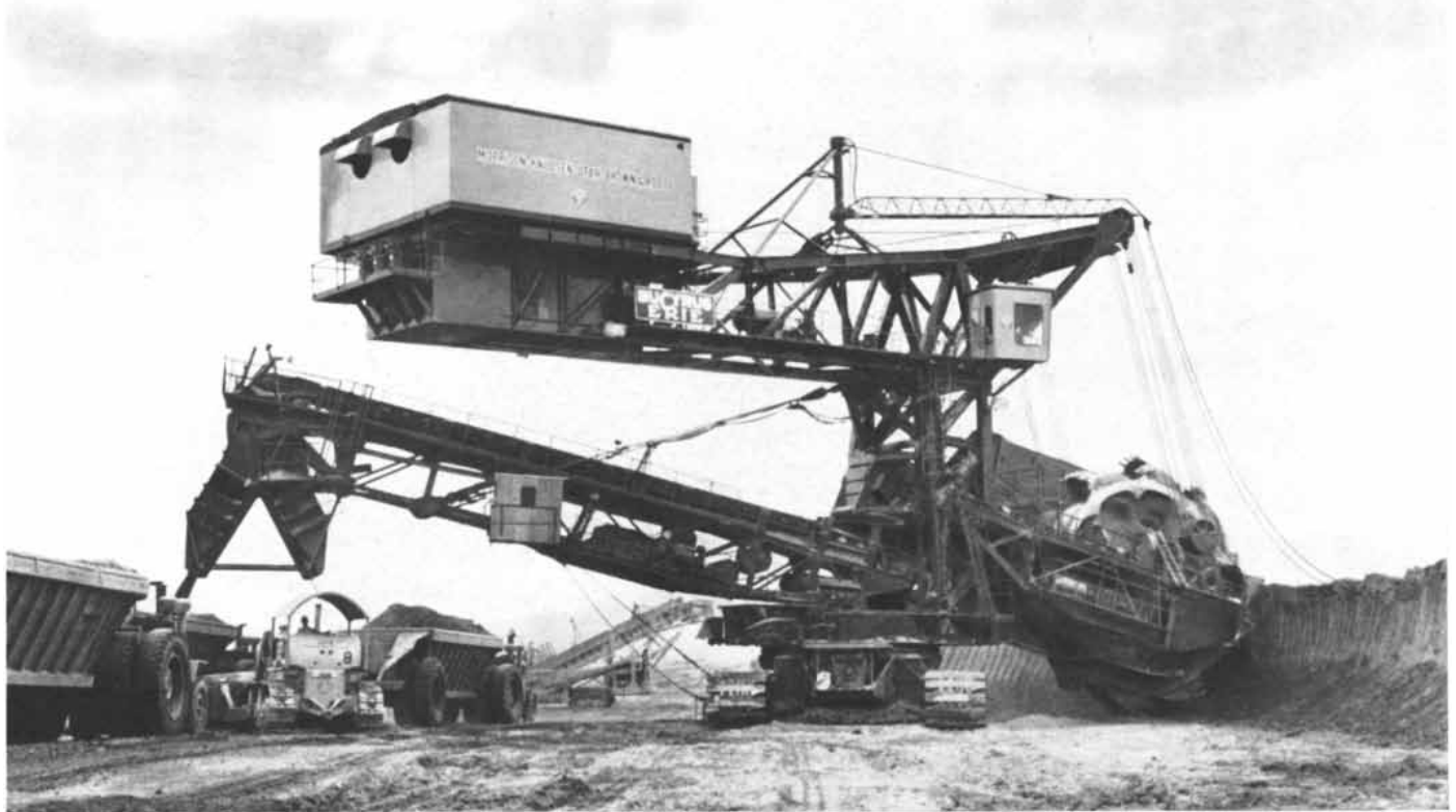
BUCKET-WHEEL EXCAVATOR is an example of the kind of machine that has been developed for rapid, large-scale surface ex-
