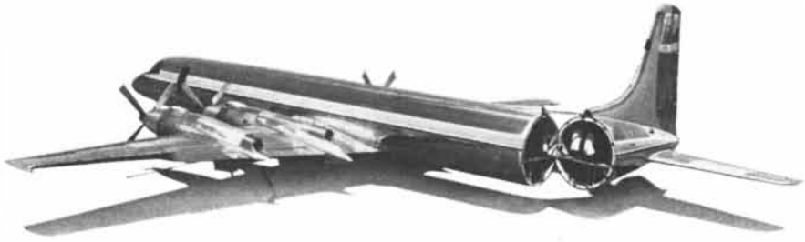
CL-44. Now carrying freight around the world. It is the first aircraft designed specifically for airfreight. The swing tail reduces loading and unloading time because of unobstructed access to the fuselage, and permits carrying longer and larger objects than possible with conventional aircraft.
