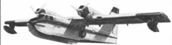
CL-215. Now in production for France and the Province of Quebec. First amphibian to be built in 30 years. Can be used for water bombing, search and rescue, patrol, cargo, crop dusting or spraying. It can scoop up about 5,500 liters of water as it taxis across a lake, take off, then drop water on fire area in an uninterrupted flight.
