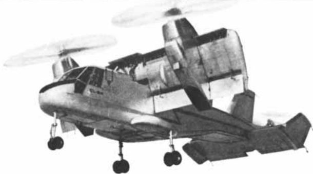
CL-84. Now in development production. It combines features of the helicopter and fixed-wing plane. With wing, engine and propeller unit tilted straight up, it can take off or land vertically. With partial wing tilt, it can take off from short fields with heavy payload. With wings and engine positioned horizontally, it can fly as fast as 300 miles per hour.
