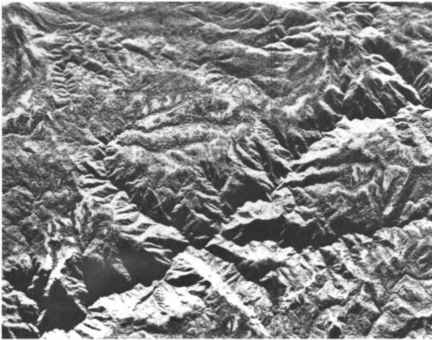
ADVANTAGE OF RADAR in penetrating a dense cover of vegetation to reveal the geologic structure of the terrain appears in a radar view of an area in the Sierra Nevada. The longer the wavelength at which radar operates, the better the radar penetrates vegetation.
