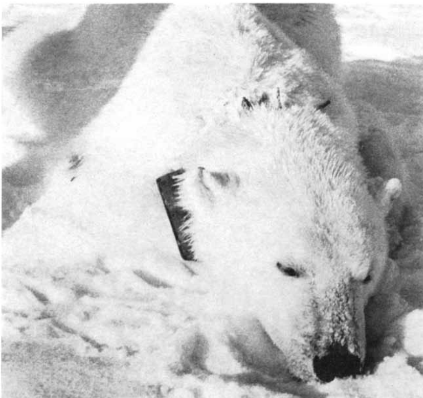
DUMMY RADIO is fastened to a collar on an immobilized bear in Alaska. The dummy matches size and weight of a radio that could be used for communication between a bear and a satellite. Experiment helped to show that a collar will stay on a bear's tapering neck.
