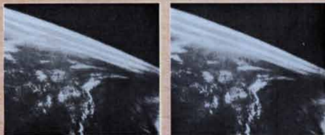
Television picture taken during GEMINI mission. Left: as originally taken. Right: reconstructed from 6:1 compressed data.
