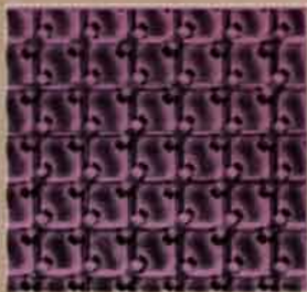
Section showing 18 mil ferrite memory cores wired in 2\frac{1}{2}D organization. Magnified 12 X.
