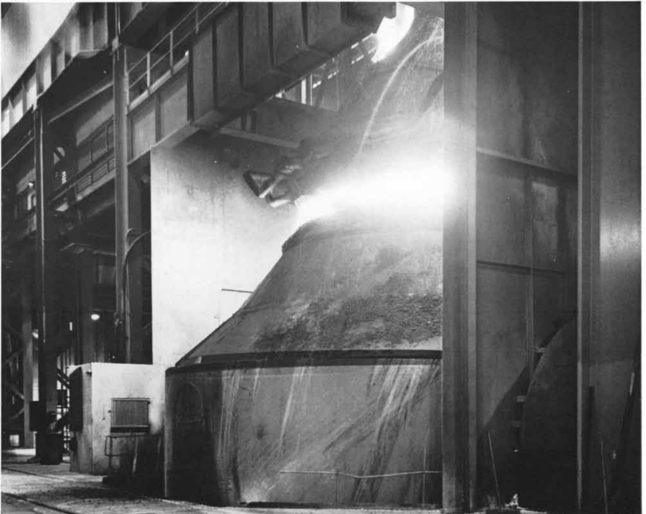
REFINING OF STEEL takes place during a "blow" in a basic oxygen furnace in the Great Lakes Steel Division of the National Steel Corporation. After the pear-shaped furnace has been tilted to receive scrap metal and molten iron it is returned to a vertical posi-
