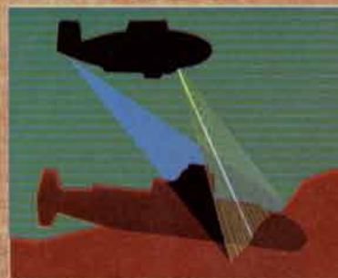
Light beamed from nose of submersible is picked up by sensor at stern.
