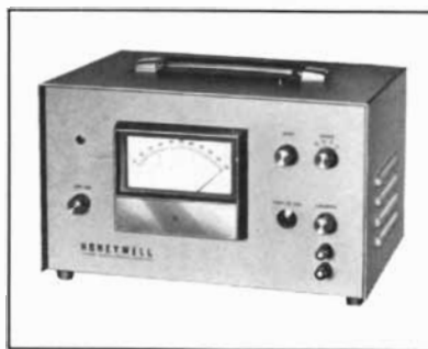
Typical hydrocarbon detector unit includes ultra-violet source, detector, sample chamber, meter and recorder output terminals.
