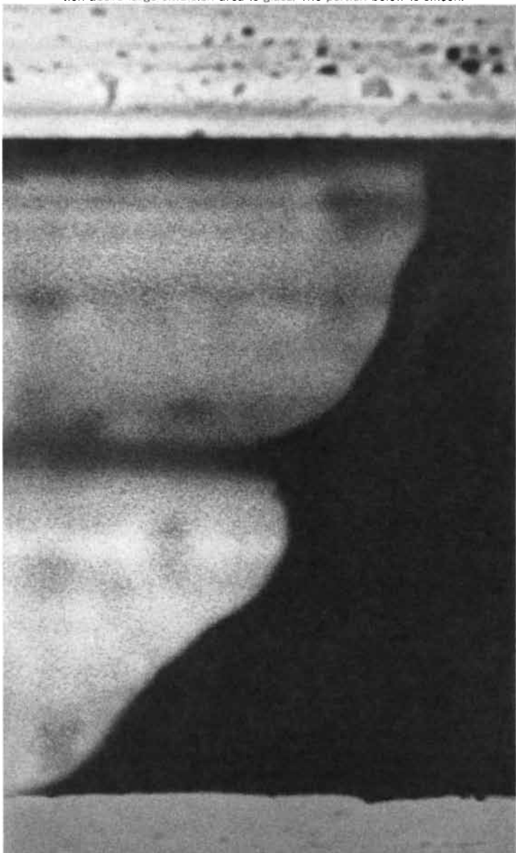
Illustration of an enlarged cross section of emulsion mask, 4 microns thick, showing ragged, sloping edge of opaque area. It is the slope of the emulsion edge that causes some fuzziness in transfer of the image to the silicon. Portion above large emulsion area is glass. The portion below is silicon.
