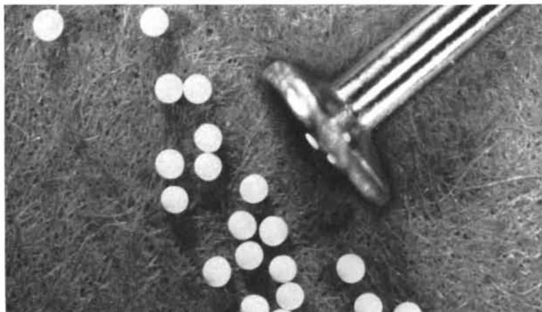
Spheres of ceramic powder, precisely formed, intimately mixed, and homogeneous—product of a new freeze-dry process devised at Bell Telephone Laboratories. A common pin indicates approximate size.
