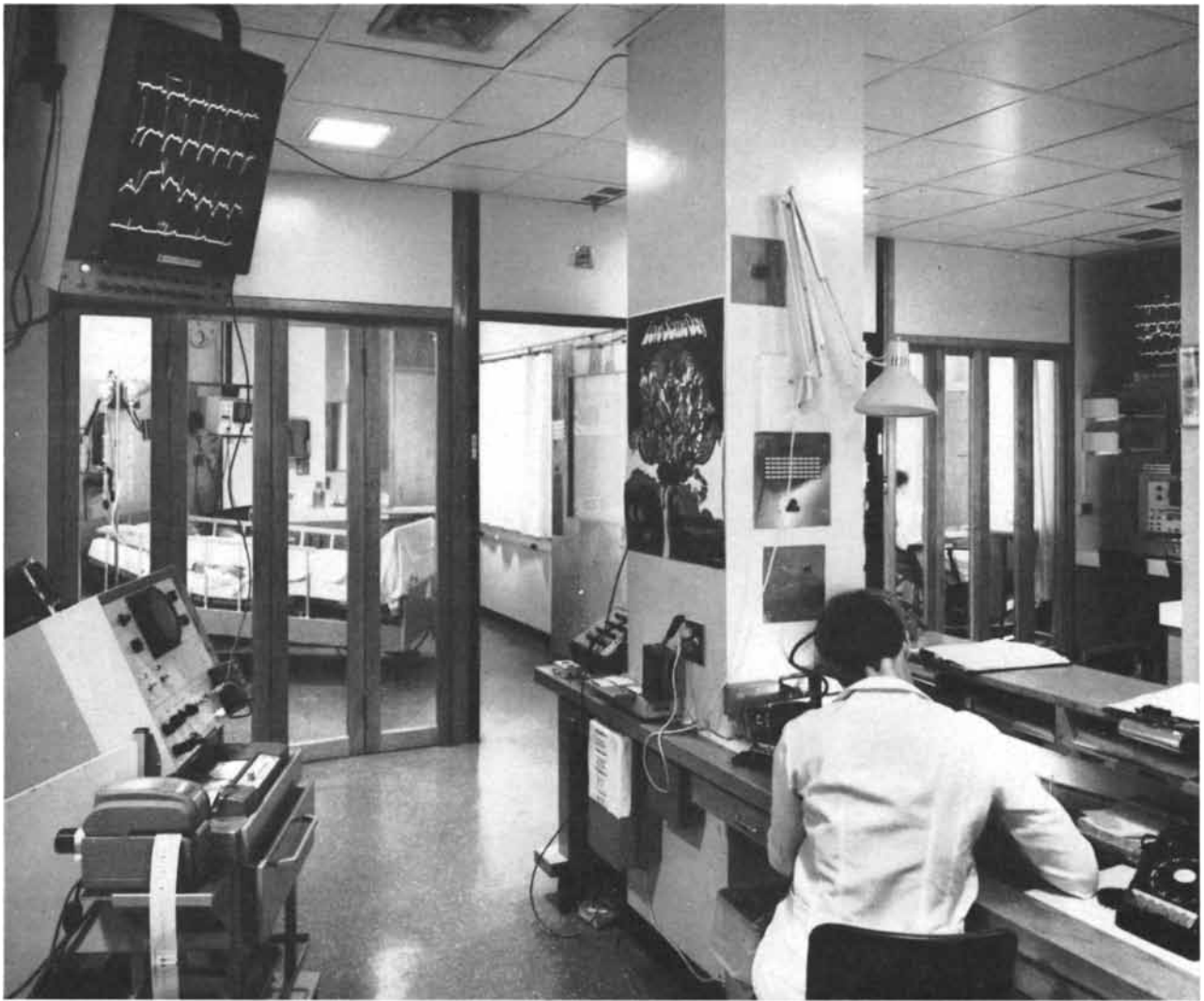
CORONARY CARE UNIT at Peter Bent Brigham Hospital is typical of several hundred such installations in U.S. hospitals. Four rooms for patients are clustered around a station from which specially trained nurses can keep a constant check not only on patients but also on oscilloscope screens that display the ECG of
