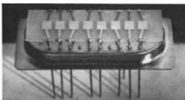
Simple monolithic filter. Input and output resonators are formed by evaporating metal areas into opposite faces of a quartz plate. The resonators are coupled through the intervening quartz. Below, in actual size, is an eight-resonator monolithic quartz filter.
