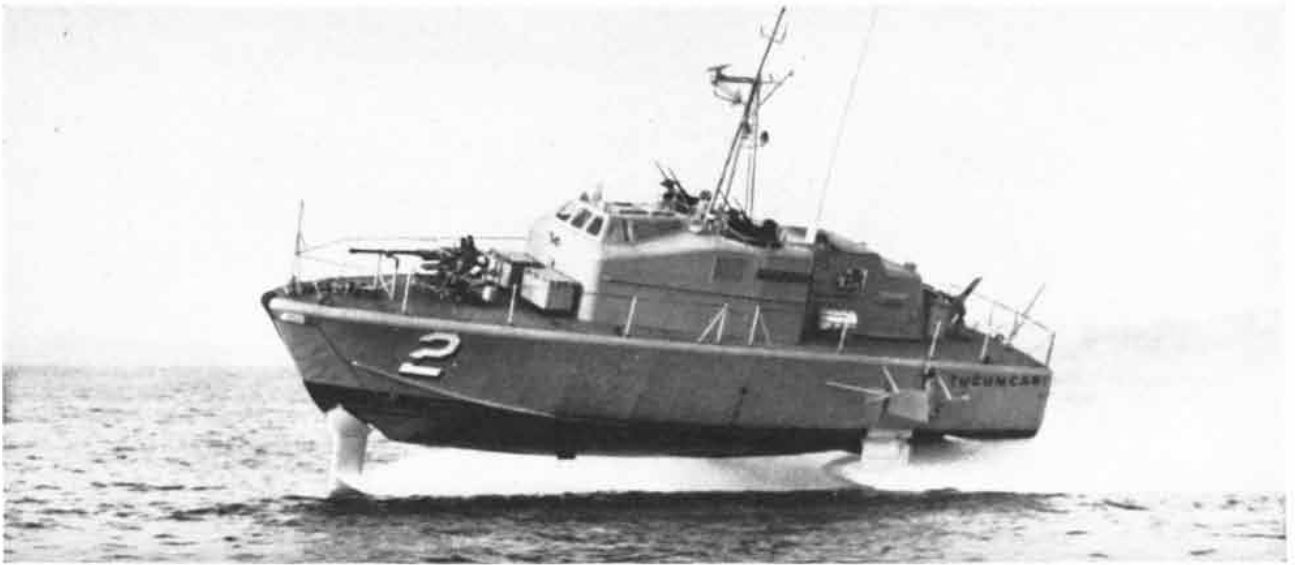
Rolls-Royce goes to sea in Boeing's new hydrofoil gunboat built for the U.S. Navy—60 tons and jet propelled. A mighty pump takes in water through the struts, spews it out the stern. Rolls-Royce supplies the power with a Marine Proteus gas turbine.
