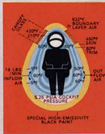
Schematic environmental diagram of SR-71 cockpit in flight conditions of Mach 3 speed at 80,000-foot altitude.
