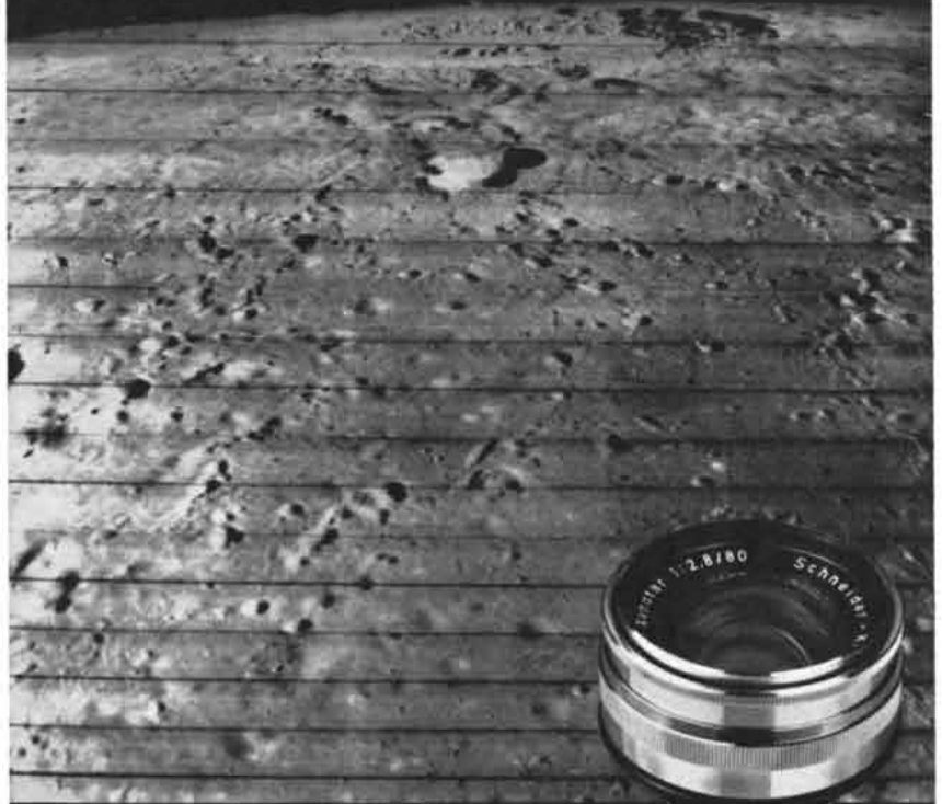
This historic NASA photo of the area near moon crater Copernicus (top center) was taken from Lunar Orbiter 2 from 23½ miles up, while surveying moon for landing sites. Lens was a Schneider 80mm wide-angle Xenotar straight from stock. Picture's high quality amazed scientists.
