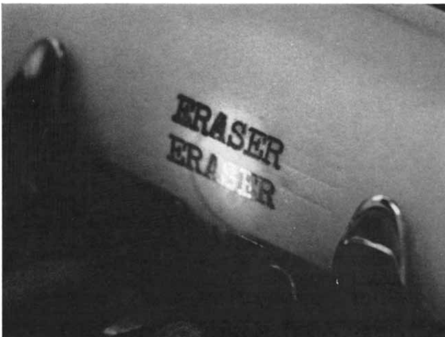
LASER ERASER invented by Arthur L. Schawlow of Stanford University is capable of vaporizing ink from paper without appreciably heating the paper. The heating of the black ink, which absorbs the laser pulse and becomes incandescent, is so rapid that the ink vapor carries away the heat before it can penetrate below the surface by conduction. The dark ring is a shadow of the end of the laser, produced by stray light from the laser flash lamp.
