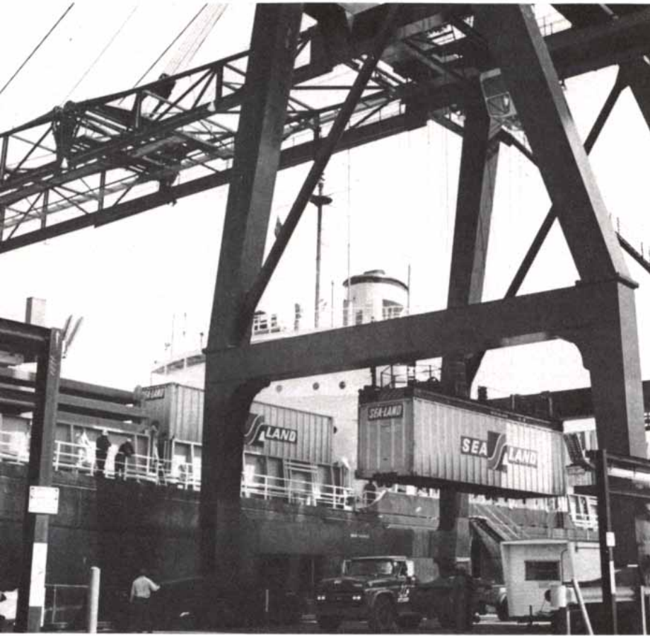
CONTAINER-SHIP STOWAGE is achieved by fitting containers into slots or grips that hold them firmly. A container ship such as this one can hold some 600 containers of this size.
