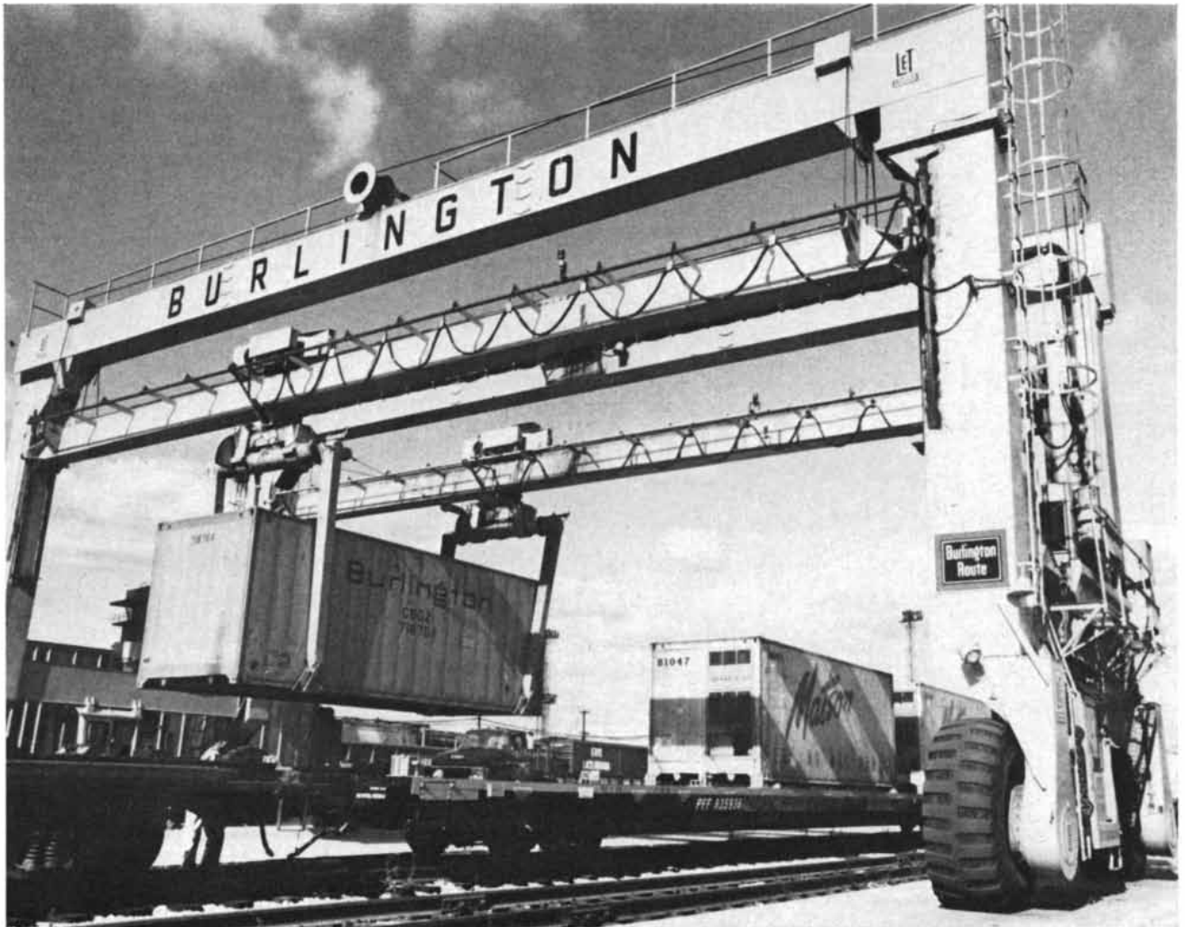
CONTAINER TRAIN of the type now being operated by a number of railroads to move only containers is loaded by a movable crane
