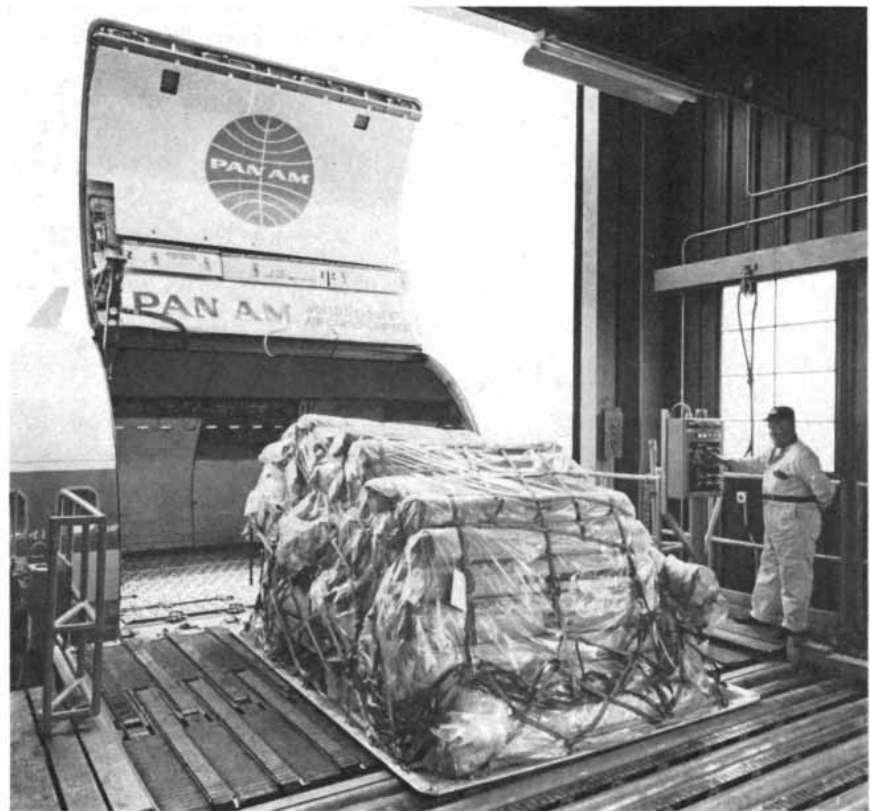
MECHANIZED PLATFORMS load cargo onto an airplane at the Pan American freight terminal. The cargo has been put on the pallet in such a way as to fit the shape of the plane.
