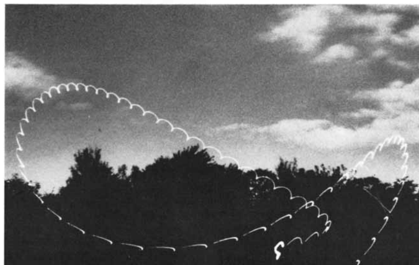
\theta -DEPENDENCE of actual boomerang orbits is demonstrated in these two moonlit photographs, in which \theta (the initial angle between the plane of the boomerang and the horizon) is about 20 degrees less in the bottom picture than it is in the top picture. The recorded paths can be compared with the theoretical paths in the middle column on page 133.
