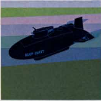
Deep Quest life-support system functions as specified in dive to 8,310 feet.
