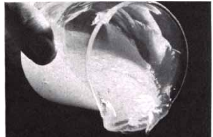
The same amount of CAB-O-SIL in dioctyl phthalate plus 20% ethylene glycol increases viscosity substantially.
