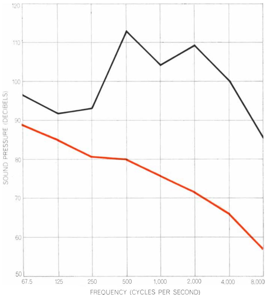
URBAN NOISE —the screech of railroad-car wheels on a sharp curve—was measured before and after a treatment consisting of a constrained-layer attachment to the flange of the wheel plus a superimposed homogeneous damping layer. The overall noise reduction was more than 25 decibels; moreover, the high-frequency components were reduced the most.
