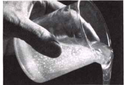
2.5% CAB-O-SIL M-5 by weight added to medium-polar dioctyl phthalate increases viscosity only slightly.
