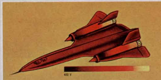
Temperature profile of the SR-71 at Mach 3+ speeds.
