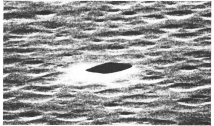
as they emit an alpha particle, are more abundant than fission tracks ( black hole, center ) but so short that they are only visible under special illumination or (as here) in a scanning electron micrograph.
