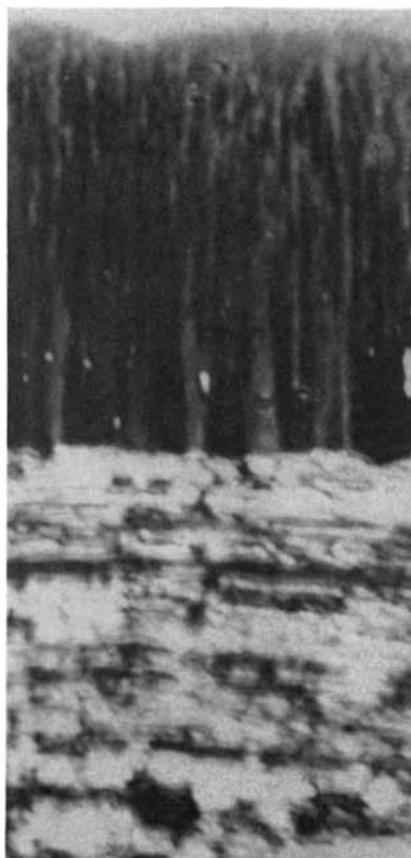
GROWTH OF COATING of silicide on molybdenum in a metal-liding process carried out at a temperature of 675 degrees C. is rapid. Coating attains a thickness of .5 mil in 50 minutes ( left ), one mil in 100 minutes ( middle ) and two mils in 200 minutes ( right ).
