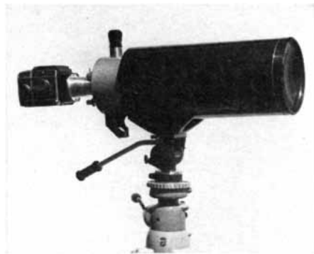
The Questar 7 with Rolleiflex FL-66 attached, mounted on the smooth-as-silk Miller Fluid Head with Lindhof Heavy Duty Tripod.
