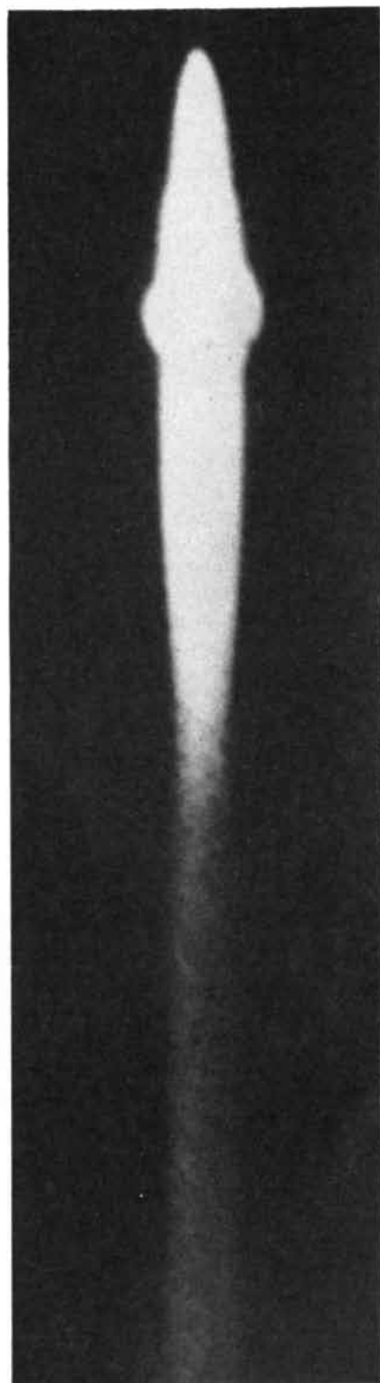
SPRINT ABM MISSILE was photographed during a test flight at the White Sands Missile Range in New Mexico. The photograph, which was released by the U.S. Army's Nike-X Project Office in March, 1966, shows the second stage of the missile heated to incandescence by friction with the atmosphere. Because of the extremely high speed of the Sprint, the missile's skin in places reaches temperatures hotter than inside its rocket motor. The bulges are created by the guidance fins at the rear of the second stage.
