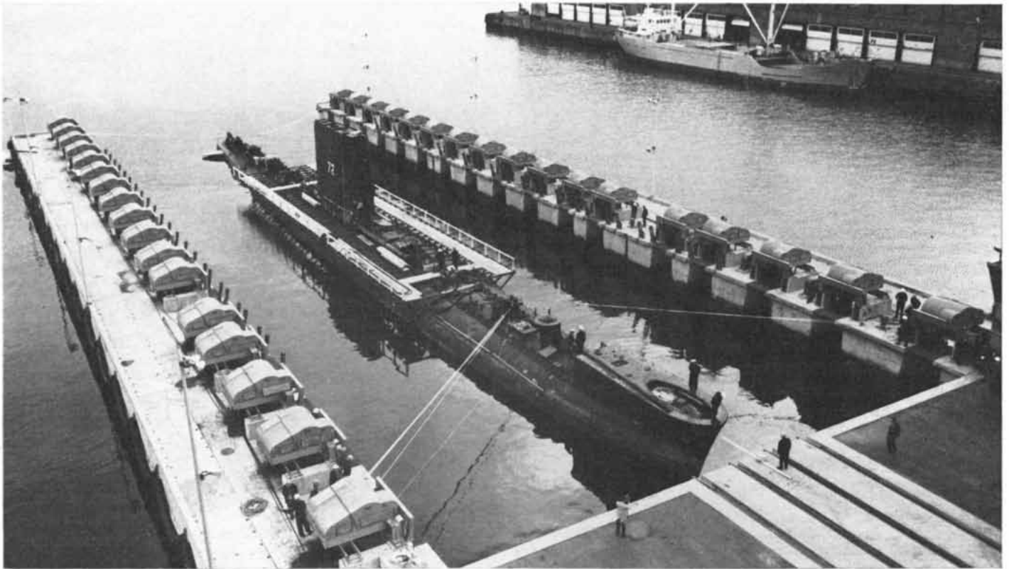
HOISTING DEVICE called the Syncrolift allows the Canadian submarine Ojibwa to be lifted out of the water ( above ) and pulled ashore on rails ( below ) for repair in a dockyard at Halifax, Nova
