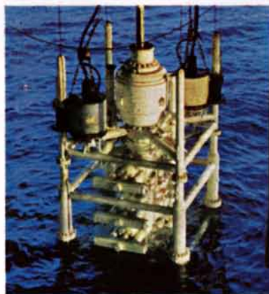
Cameron highly-specialized wellheads and blow-out preventers for underwater drilling.
