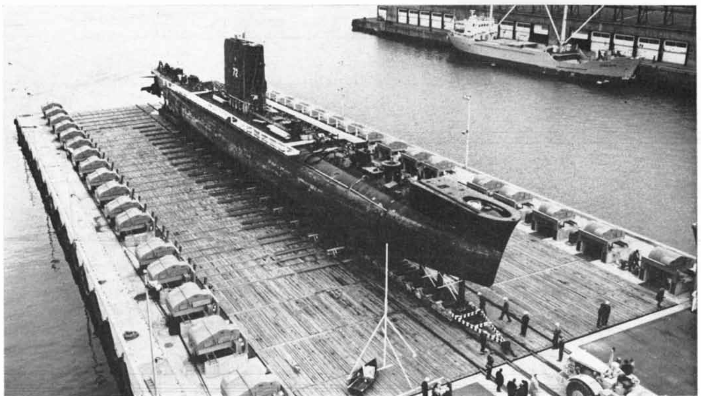
HOISTING DEVICE called the Syncrolift allows the Canadian submarine Ojibwa to be lifted out of the water ( above ) and pulled ashore on rails ( below ) for repair in a dockyard at Halifax, Nova
