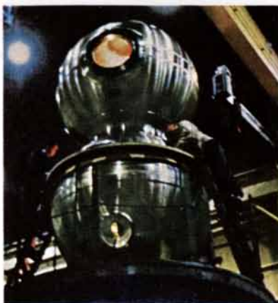
Cameron vacuum-melted alloys for bi-spherical pressure hull for the 8000' operating Deep Quest.
