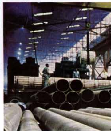
Cameron heavy wall extruded pipe for pipelines and offshore platform supports.
