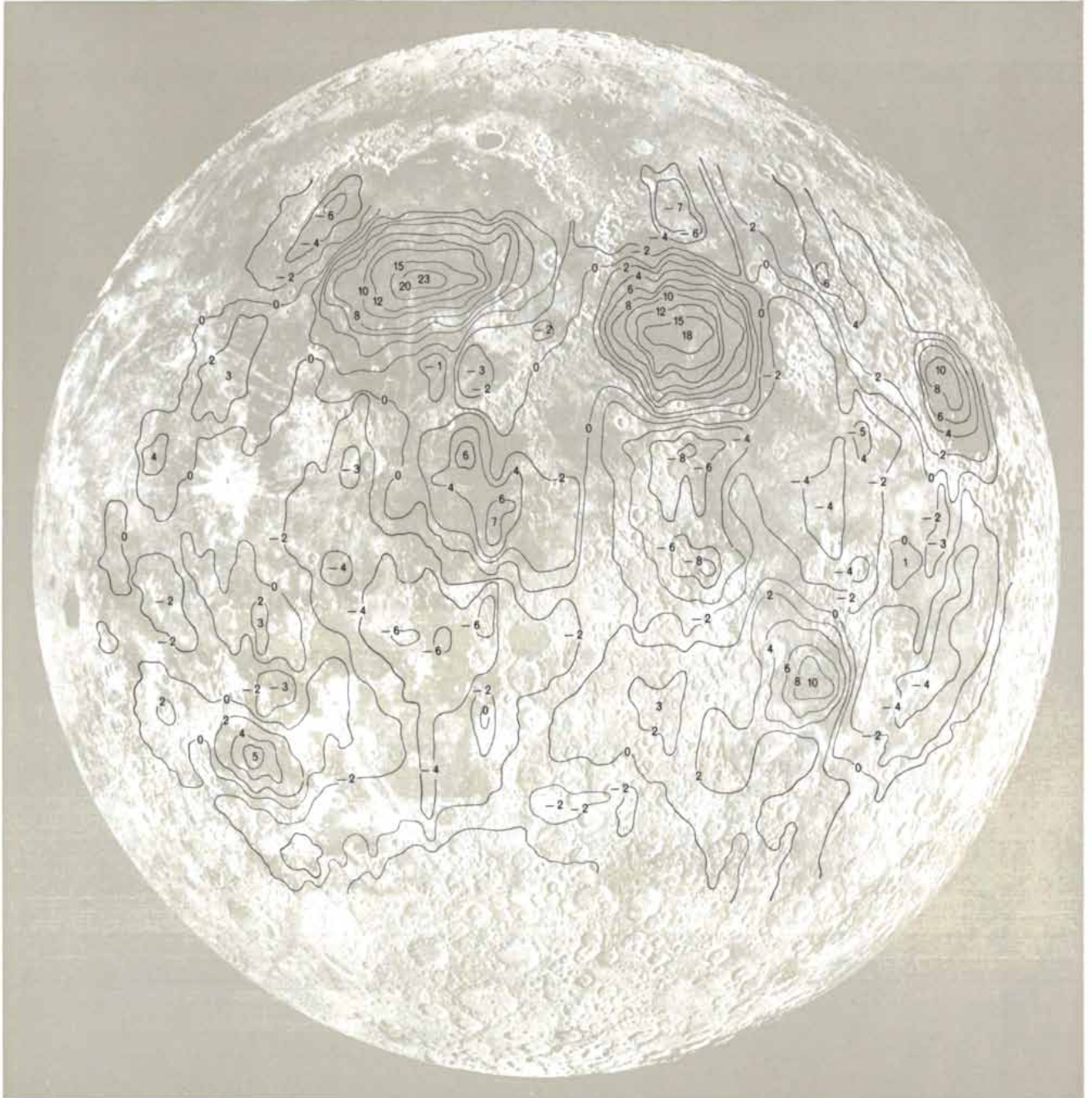
MASS CONCENTRATIONS revealed by perturbations in the orbits of spacecraft orbiting the moon are represented by contours showing gravitational acceleration in tens of milligals. One milligal
