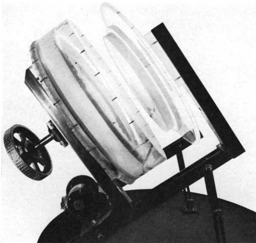
SEPARATED PARTS of the model basin reveal the configuration whereby the water is held in the shape of a segment of the surface of a sphere, which is the ocean's configuration. Bottom block is convex and top one concave; their normal separation is one centimeter.
