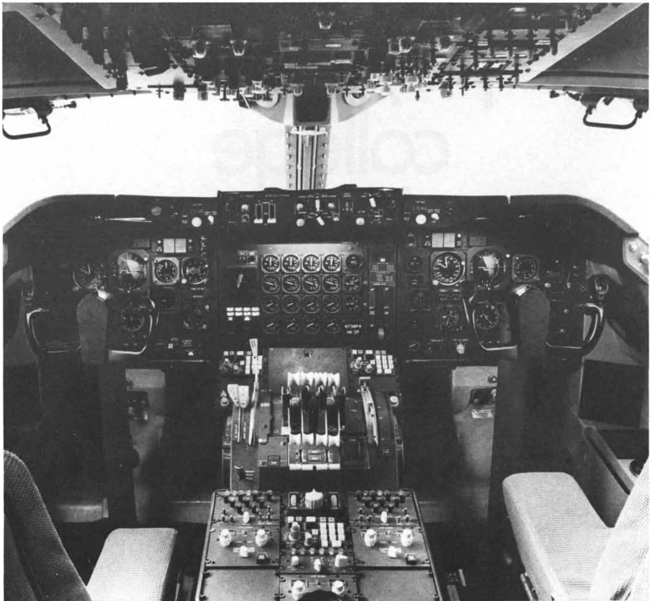
INSTRUMENT PANEL of a Boeing 747 commercial passenger aircraft includes the control and display devices associated with three complete Carousel IV inertial-navigation systems ( bottom
