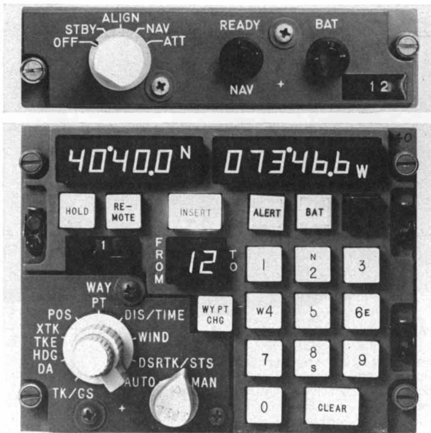
PILOT'S CONTROLS for Carousel IV, an inertial-navigation system manufactured by the AC Electronics Division of General Motors Corporation, are shown. Device at top is called the mode-selector unit; one at bottom is the control and display unit. Abbreviated settings are STBY (standby), NAV (navigate), ATT (attitude), BAT (battery), TK/GS (track/ground speed), DA (drift angle), HDG (heading), TKE (track-angle error), XTK (cross-track distance), POS (position), WAY PT (way point), DIS (distance), DSRTK/STS (desired track/status), AUTO (automatic), MAN (manual), WY PT CHG (way-point change).
