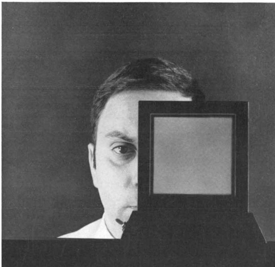
LIQUID-CRYSTAL WINDOW can be made opaque at the flick of a switch. The window consists of two glass plates enclosing a layer of liquid crystal. Transparent electrodes of tin oxide coat the inside surfaces of both plates. At top the pane is clear, and the man's face can be seen clearly because the device has not been turned on. At bottom a voltage has been established across the electrodes and the electric field creates turbulence in the liquid crystal. The turbulent areas make the pane opaque; accordingly the man's face is obscured.
