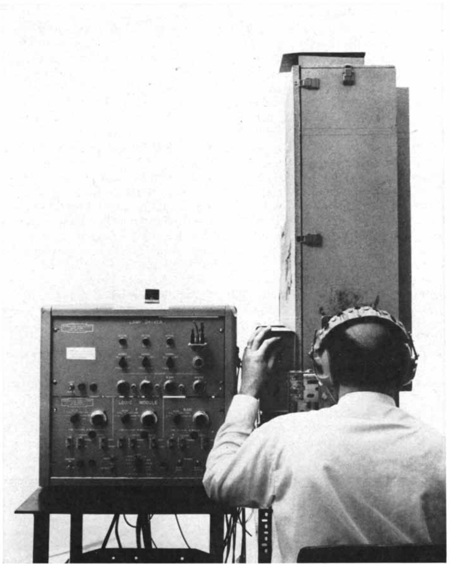
TACHISTOSCOPE ( tall box at right ) is a viewing chamber in which an experimental subject watches rapidly changing stimuli such as images or light flashes. Apparatus at left controls timing and presentation of the stimuli. The subject also wears earphones through which he hears clicking sounds. He controls the tone generator that produces the clicks so that one coincides with the onset of an image and the other with the termination. Such experiments reveal how the memory processes letters, numbers and similar material.
