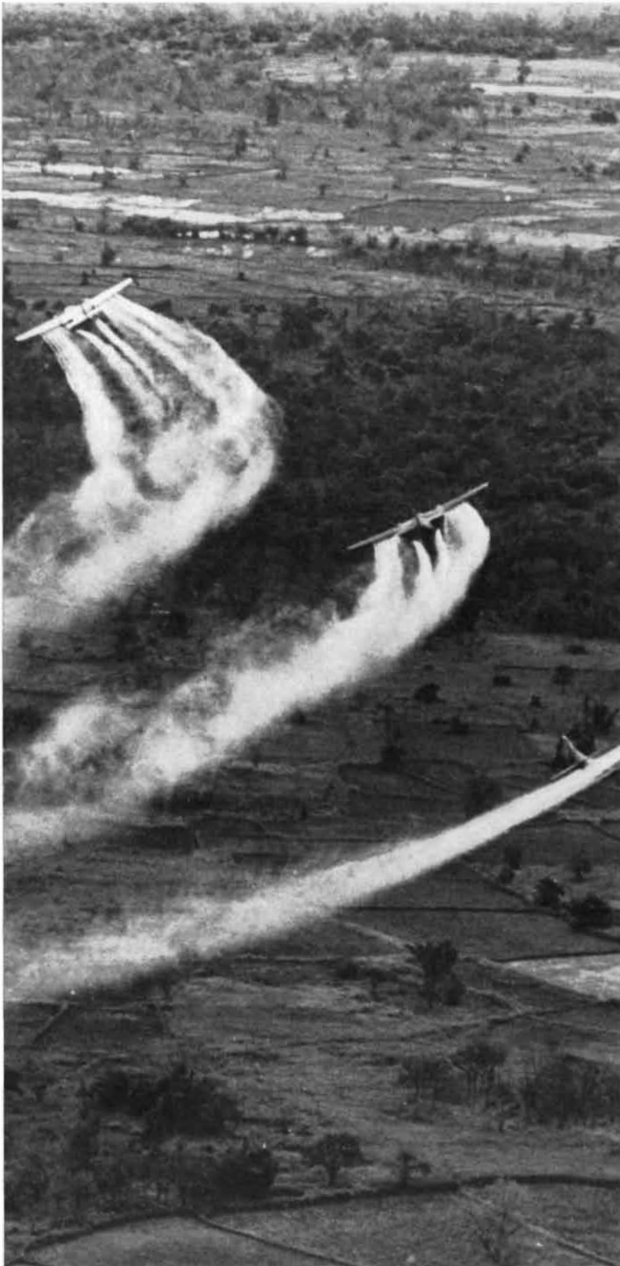
HERBICIDES ARE SPRAYED by U.S. Air Force planes in South Vietnam. More than 19,000 sorties have been flown since 1962. One aircraft covers a swath nearly 300 feet wide and 10 miles long. Military officials say destruction of crops in certain areas held by Vietcong reduces food supplies for opposing forces and jungle defoliation reduces concealment.
