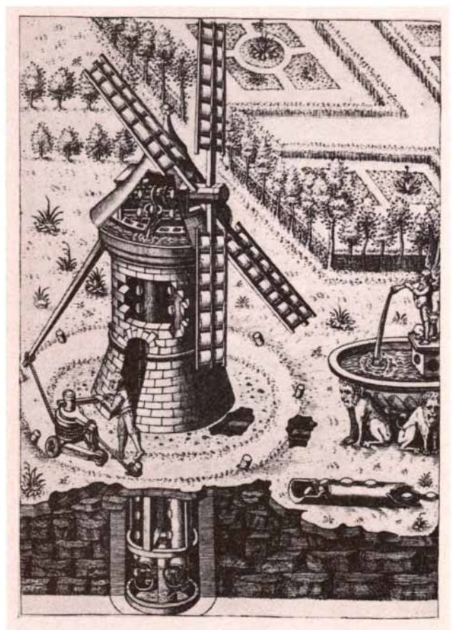
SECOND WINDMILL , with a horizontal axle, was invented independently in the 12th century in the North Sea region of Europe. The one shown is a "tower mill." Only its top is turned to the wind.
