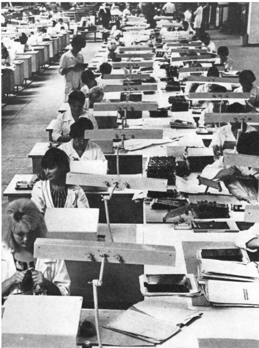
COMPUTER FACTORY IN KIEV makes both general-purpose computers and process-control computers, such as the Dnepr-2. Here workers are assembling electronic components on printed circuit boards, a technique characteristic of second-generation machines.
