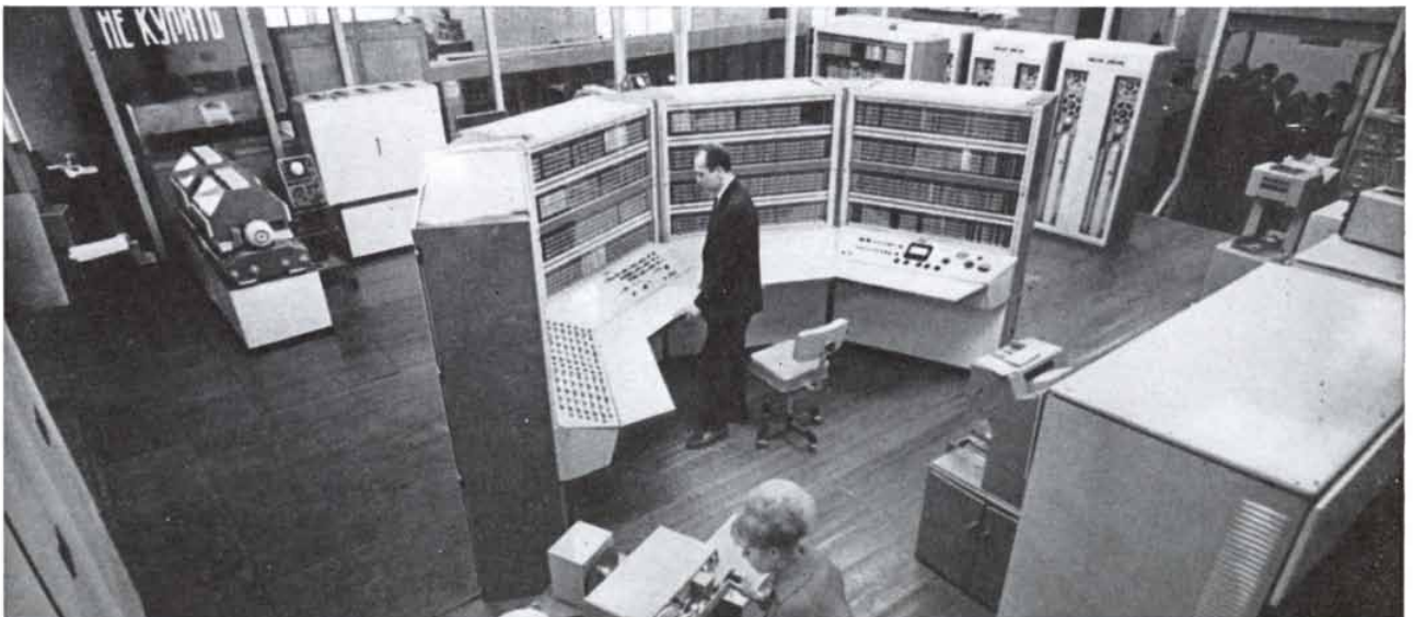
LARGEST RUSSIAN COMPUTER , the BESM-6, compares favorably with all but the most powerful American machines. The BESM-6 can perform about a million operations a second. Current models have storage space for 65,000 words, each 48 data bits in
