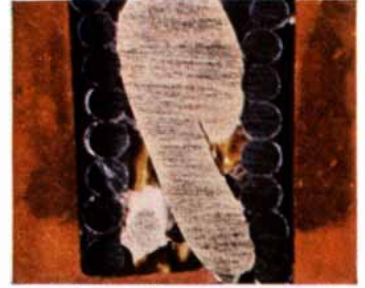
Macrophotographic section of wire nut. Polacolor Type 58 film.
