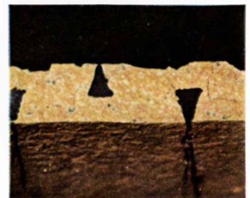
Macrophotographic section of battery grid. Polacolor Type 58 film.
