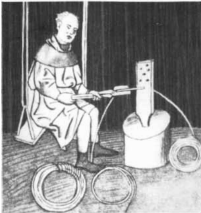
Medieval German "schockenzieher" (shock drawer) pulled wire through die by swinging back and forth.
