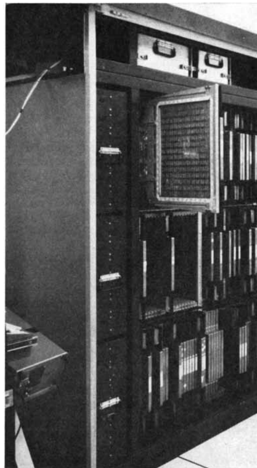
COMPUTER ILLIAC IV is nearing completion at the Great Valley Laboratories of the Burroughs Corporation in Paoli, Pa. Unlike conventional computers, which carry out logical and arithmetical operations in
