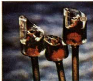
Macrophotograph, diode fractures
