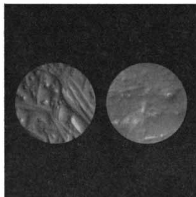
Surface of original ceramic (left), and, (right), with finer grade of silica.
