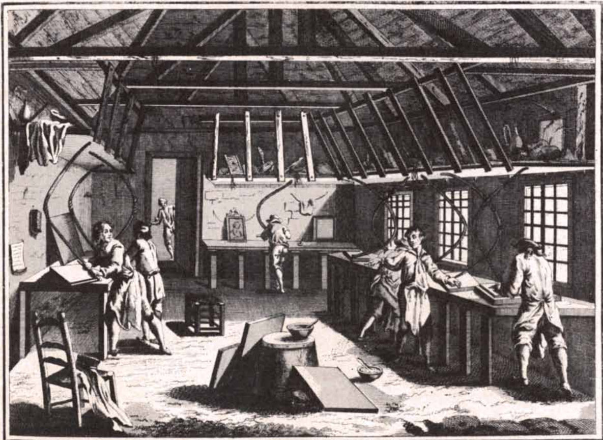
MEASURE OF MUSCLE POWER was made in 1699 by Guillaume Amontons of the Paris Academy of Sciences with men who polished glass. A pad, pressed against the glass by a bow, was pushed
