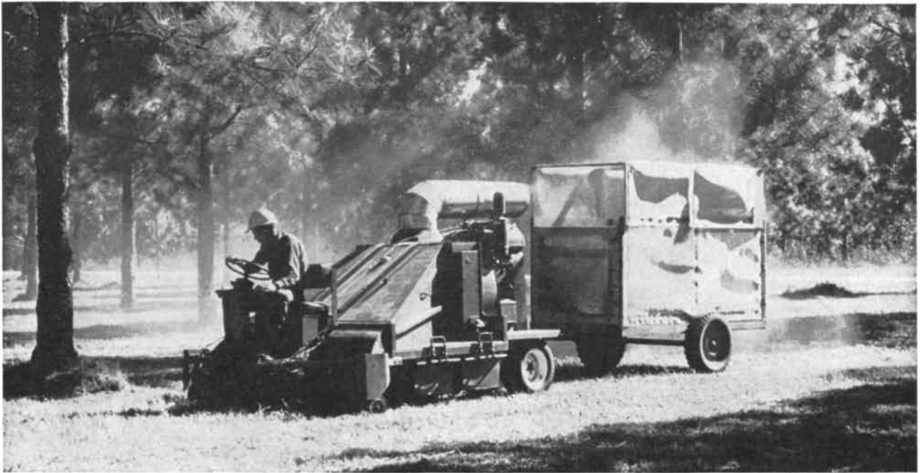
VACUUM SWEEPER is being developed by the North Carolina Tree Improvement Cooperative for collecting seeds that have fallen to the ground in a seed orchard. The machine is designed for
