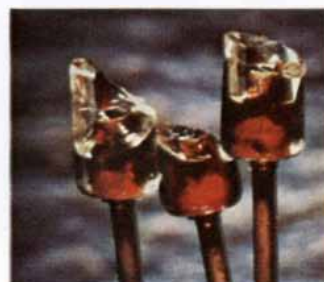
Macrophotograph, diode fractures
