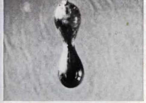
Glass bead from Apollo 11 lunar soil 100x Dr. W. D. Ehmann, University of Kentucky
