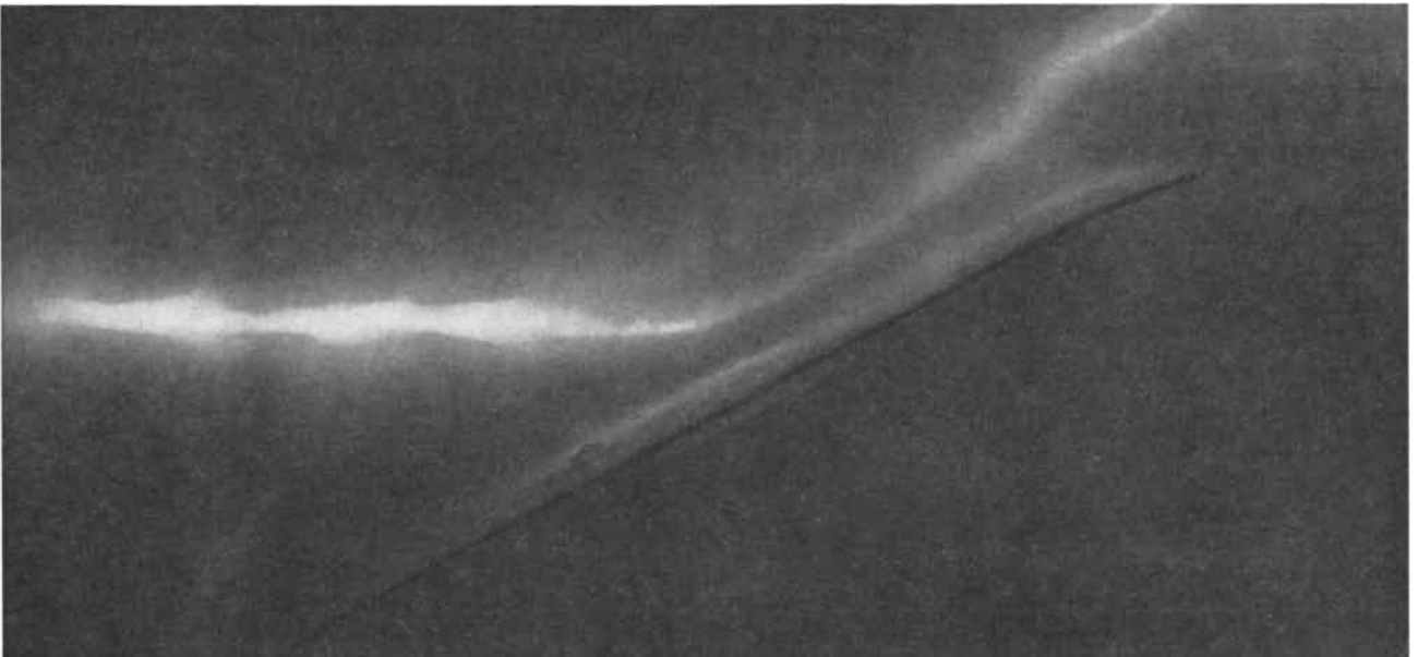
CURIOUS BEHAVIOR of a very intense, high-energy electron beam in a low-pressure gas is captured in this photograph, also from Physics International. When a tilted metal plate is placed in the
