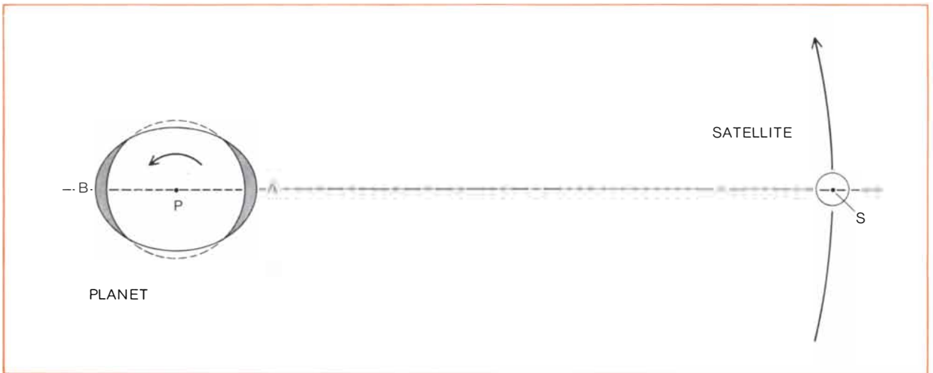
TIDAL DISTORTION at the equator of a perfectly elastic planet is caused by a satellite traveling in a circular orbit. The gravitational force of the satellite would deform the planet into an ellip-
