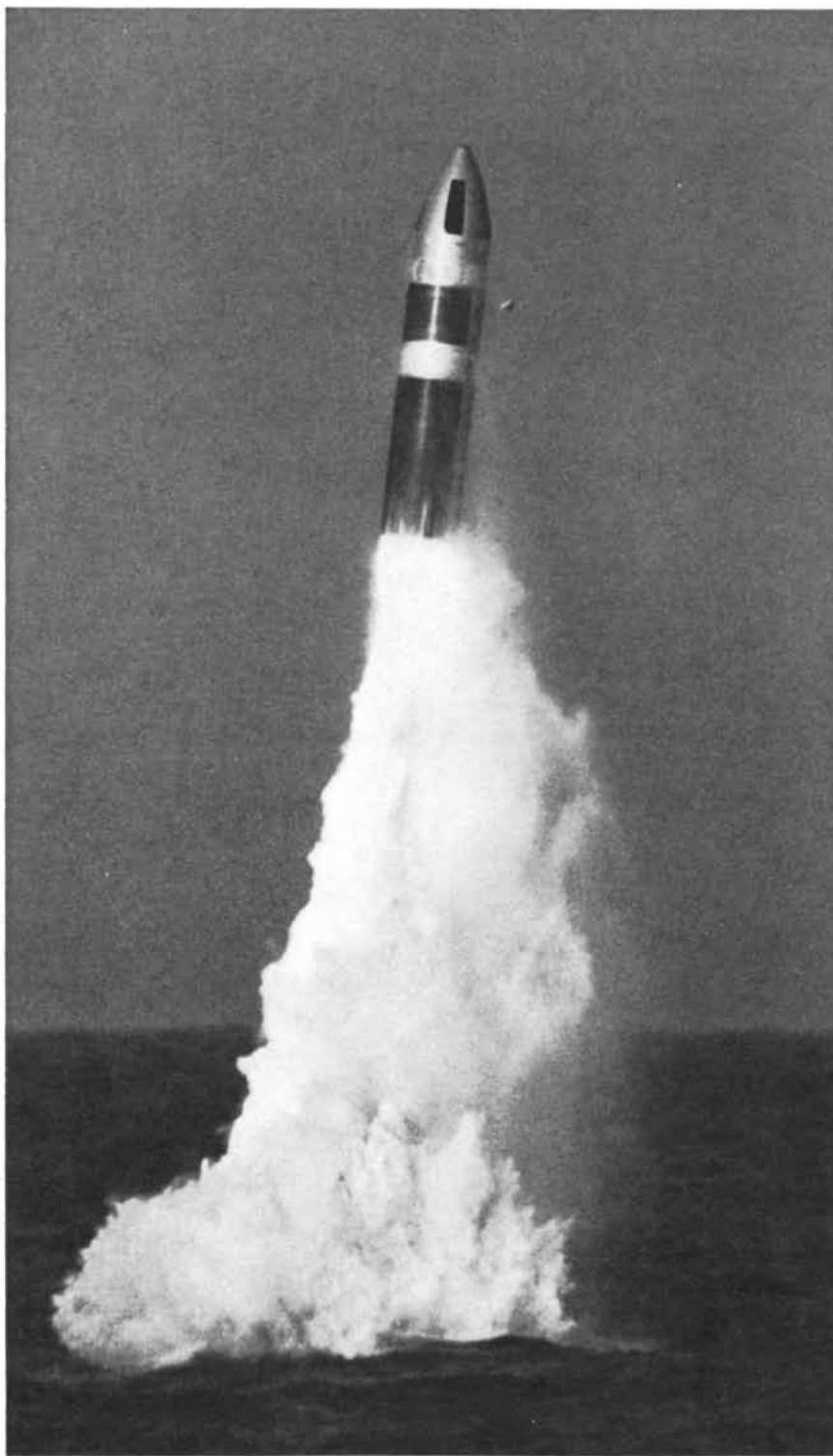
FIRST SUCCESSFUL TEST LAUNCH of a Poseidon missile from a submerged submarine was carried out in October, 1970. The missile was launched from the James Madison . The Poseidon missile, like the earlier Polaris models, is expelled from its silo by compressed gas; its rocket engine is then ignited after the missile has cleared the surface of the water.
