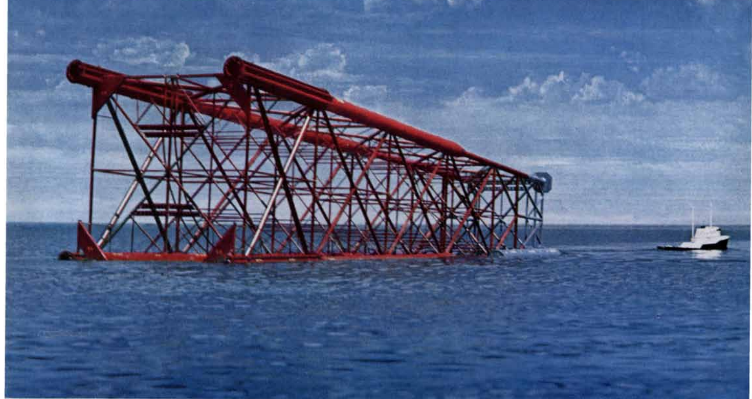
This is a sixteen-foot model of what someday may be the tallest offshore platform. It will be nearly as tall as the Empire State Building, but only the tip will rise above water. The model was used to determine how such a huge structure can be safely towed and submerged in place.
