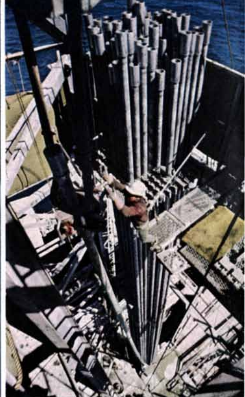
(Left) Helicopters carry small equipment and men to the rigs. Crews work seven days on, then have seven days off. (Right) To replace a worn bit, the entire drill pipe is taken apart, stacked in the derrick, and then reassembled. Drillers call this oft-repeated cycle "making a roundtrip."
