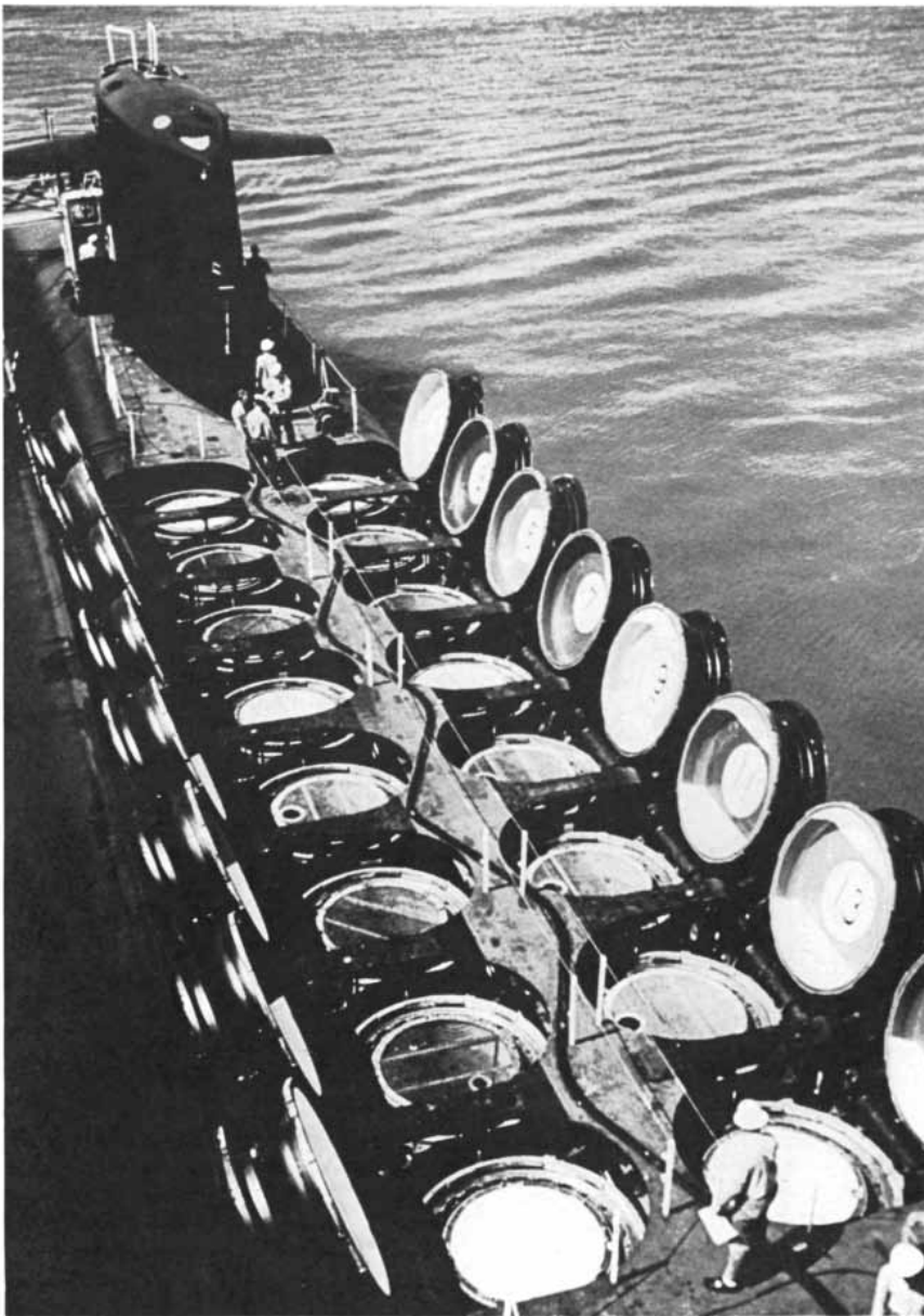
ARRANGEMENT OF MISSILE SILOS in a Lafayette-class Polaris submarine is revealed by the open silo doors in this view. The submarine, the U.S.S. Sam Rayburn , was photographed at Newport News, Va., at about the time of her commissioning in December, 1964.
