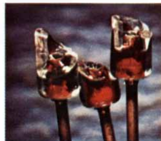
Macro photograph, diode fractures
