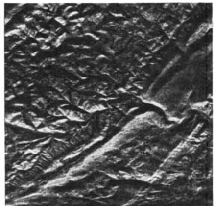
DEPTH REVERSAL occurs when some pictures are viewed upside down because the eye assumes that light is coming from the top. The valleys and ridges in the picture on the left (an aerial side-looking-radar view of the Appalachians) turn into ridges and valleys (right).
