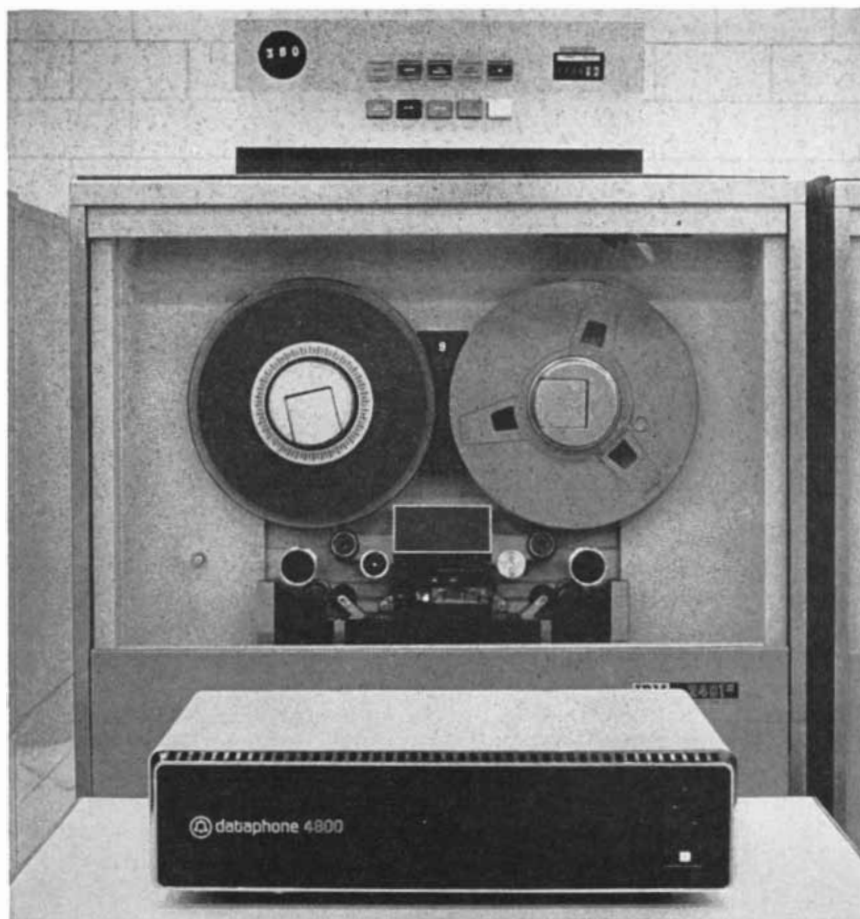
BELL SYSTEM MODEM converts digital data from business machines and computers to an analogue signal well adapted for traveling over a telephone voice channel. The modem is the oblong box in the foreground; in the background is part of the computer. In this modem the phase of a carrier wave is rotated by one of eight allowed amounts, thus tripling the channel bit rate over the rate provided when only two phase changes are used. An adaptive filter automatically compensates for the "pulse-smearing," or dispersion, that the signal may suffer in transmission. The modem operates at the rate of 4,800 bits per second.
