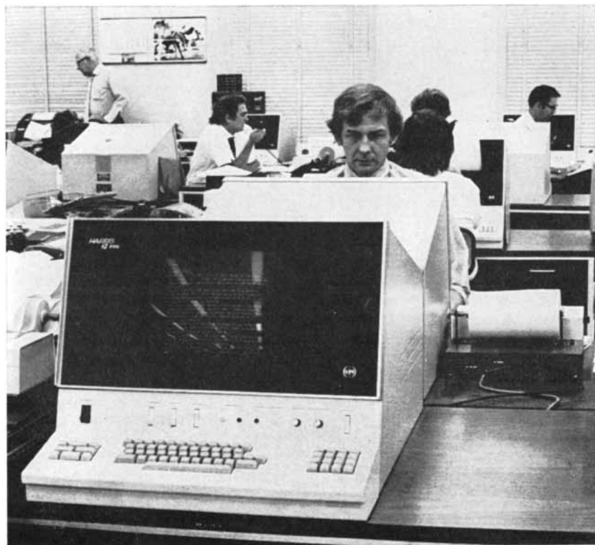
EDITING AND PROOFING TERMINAL built by the Harris-Intertype Corporation is representative of an extensive family of computer terminals that combine a keyboard with a pictorial display. The terminal is designed to be the primary means of correcting, editing and proofreading text prior to typesetting. It can accept data from a computer or paper tape at the rate of 1,200 characters per second. Once the copy has been edited the terminal can produce a tape output or transmit the text to a computer for subsequent typesetting.
