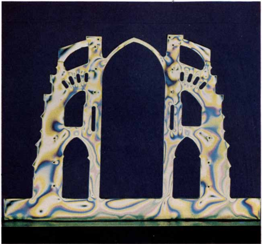
CHARTRES MODEL , stressed by simulated wind loading, is of a section across the nave of the cathedral. The pattern can be interpreted as a contour map of stress intensity; each color represents a different order of interference, which is related to intensity of stress. The stress is zero in black regions of the model and is highest where fringes are closely spaced.
