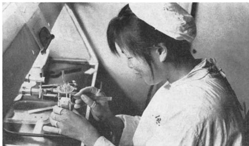
PHOTOMULTIPLIER, an important research tool, is being assembled by a young worker in a university workshop. Self-sufficiency in such equipment is a major goal in China now.
