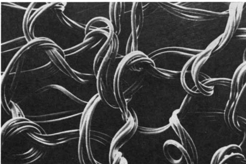
EFFECT OF TEXTURING is to give yarns increased bulk, fuzziness or stretchability. The double-knit fabric ( top ) is made with a textured polyester yarn; note the waviness of the filaments. The woven polyester fabric ( middle ) has a textured filling (horizontal yarn) and untextured warp. The stretch hosiery ( bottom ) is knitted of a textured nylon yarn.
