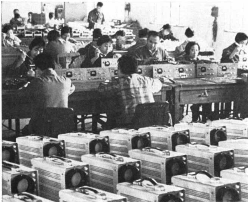
PORTABLE OSCILLOSCOPES manufactured in this workshop are lined up on the table; they appear to be simple instruments, probably suitable for use in the field. Electronic equipment is manufactured in China in factories, technical institutes and even universities.
