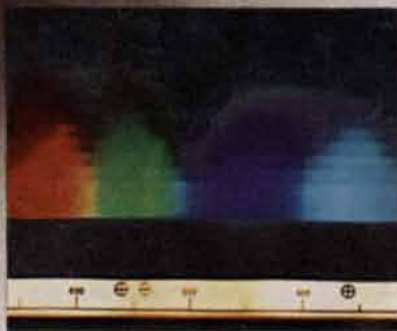
Spectrogram of xenon flash tube emission.
