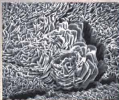
Scanning electron micrograph of zinc crystals on galvanized iron.
