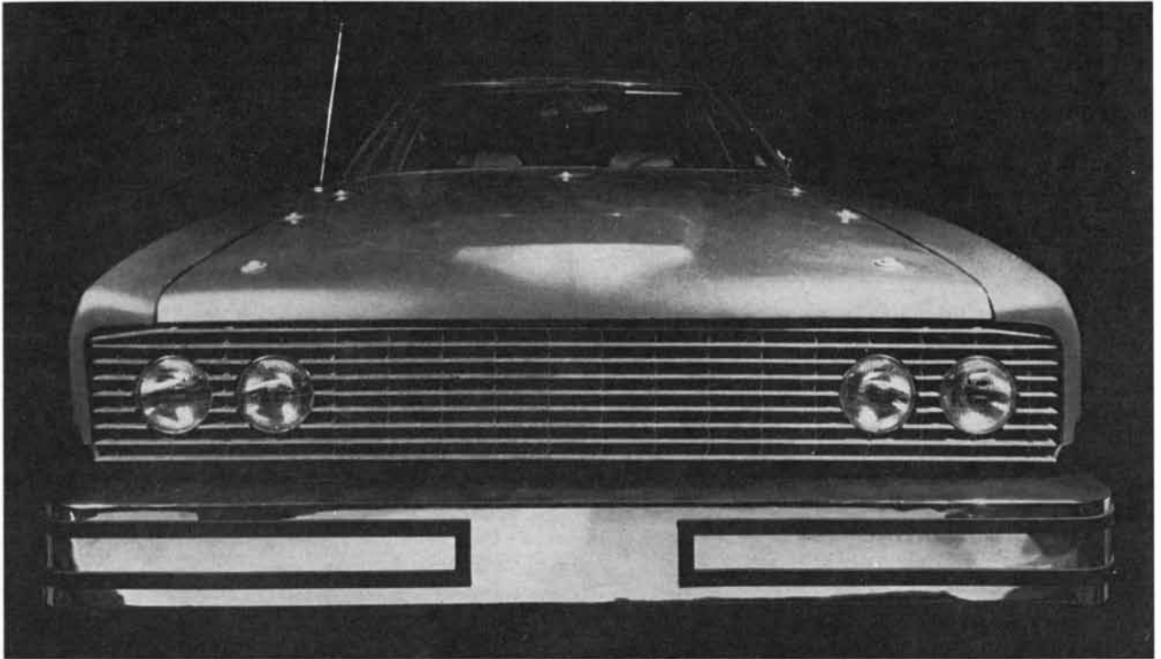
FRONT-END MODIFICATIONS designed by the Calspan group include a strong bumper made of high-strength steel and backed
