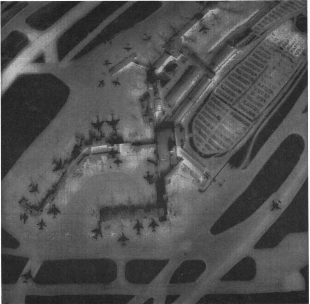
INFRARED PHOTOGRAPH of an airport in Texas was made from an aircraft flying at an altitude of 2,000 feet. Since infrared photography is not dependent on the sun for illumination, it is used in reconnaissance satellites for night applications or in polar regions.
