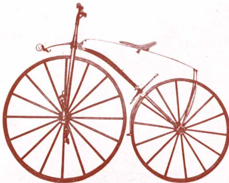
FRENCH VELOCIPEDE , produced by Pierre and Ernest Michaux in Paris in 1863, was the first commercially important machine on the way to the modern bicycle. The "bone-shaker," as the vehicle was sometimes called, had cranks with pedals fixed directly to the hub of the front wheel and hence suffered from the limitation of having too low a gear ratio.
