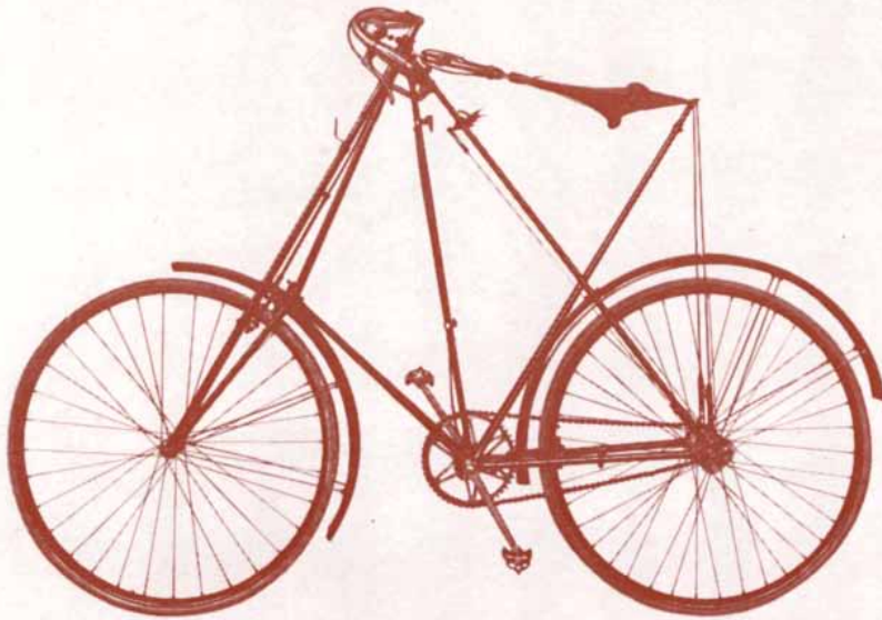
FULLY TRIANGULATED FRAME was the most distinctive feature of the Dursley-Pedersen bicycle, which achieved some success in England in the 1890's. This machine used small-diameter tubes in pairs and was remarkably light, weighing in at only 23 pounds.
