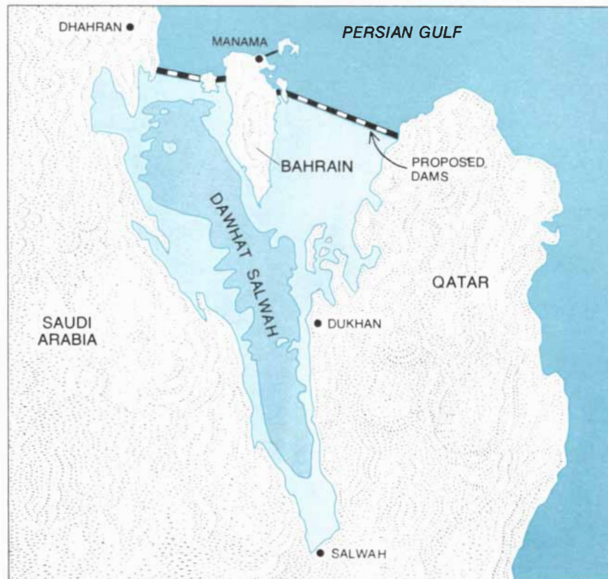
SCALE of the heliohydroelectric project advanced by Kettani and Gonsalves is suggested by the map of the entire Persian Gulf area at top and by the more detailed map at bottom. The total surface area of the proposed reservoir (lighter shades of color) would be 6,460 kilometers. The marginal lands that could be reclaimed from the sea in Dawhat Salwah, amounting to some 4,100 square kilometers, are indicated in the lightest shade of color.
