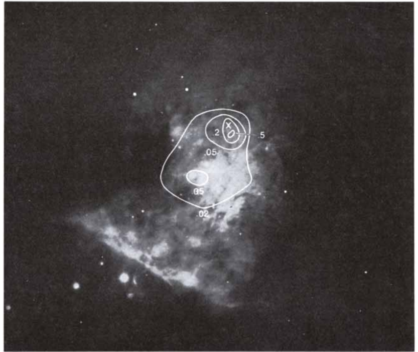
TWENTY-MICRON FLUX IN ORION NEBULA is superposed on a photograph taken at the Lick Observatory. The innermost contour is equal to half the 20-micron flux of Betelgeuse as measured with an aperture of five arc seconds. The outermost contour equals a fiftieth the flux of Betelgeuse. Trapezium stars are within lower .05 contour. X denotes a point source that seems to be a protostar with a surface temperature of about 600 degrees K.
