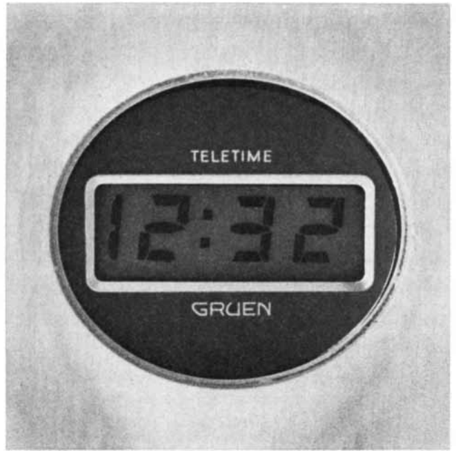
poration. Watch on the right, made by Gruen Industries, Inc., has field-effect liquid-crystal display made by the International Liquid Xtal Company. Both systems operate by reflecting ambient light.
