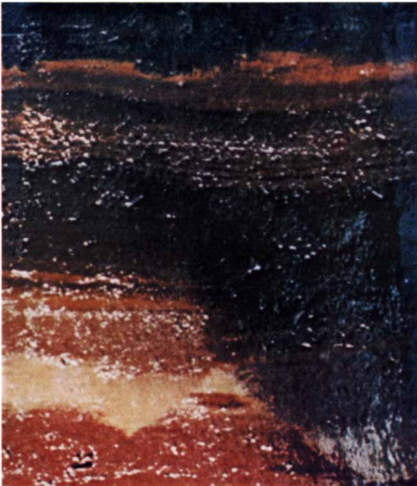
METAL-RICH CORE , collected from the Atlantis II Deep, one of the hot-brine pools located along the axial valley of the Red Sea at a depth of about 6,600 feet below sea level, represents the most concentrated submarine metallic sulfide deposits known. The muddy sediments containing the sulfide minerals fill the Red Sea basins to a thickness estimated at between 65 and 330 feet. The deposits are saturated with (and overlain by) salty brines considered to be the hydrothermal solutions from which the sulfide minerals were precipitated. The photograph was made by David A. Ross of the Woods Hole Oceanographic Institution.
