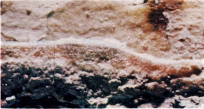
SMALL VEIN OF PURE COPPER was discovered in a core sample of sedimentary rock obtained by the Deep Sea Drilling Project some 350 miles southeast of New York City. The copper vein, the horizontal reddish structure in this longitudinal section of a piece of the original core, is about half an inch long. It was found in sediment about 65 feet above the volcanic basement rocks under the lower continental rise at a water depth of 17,000 feet.
