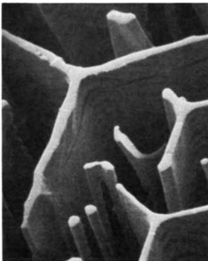
IRREGULAR STRUCTURE of this experimental eutectic composite, developed by G.E., is evident in the sequence of successively enlarged scanning electron micrographs shown here. The fiber material, tantalum carbide, is the same as in the micrograph on page 37; the difference in the form of the fibers results from the use of a different matrix alloy, in this case pure cobalt.
