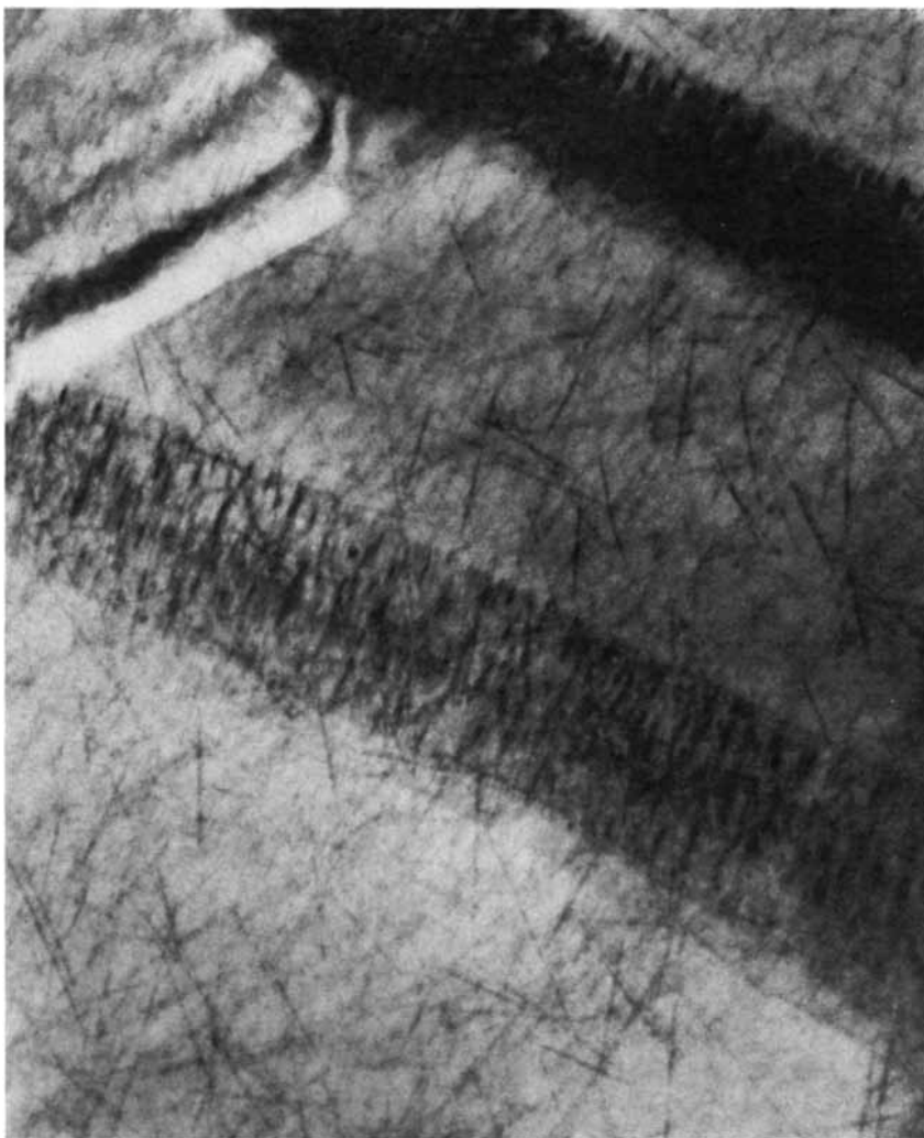
NUCLEAR TRACKS in a crystal of the Fayetteville meteorite, which show up as the thin, short dark lines, were formed by the nuclei of iron and some heavier elements. They were photographed at a magnification of 60,000 diameters with a high-voltage electron microscope by David J. Barber and P. Buford Price, Jr., of the University of California at Berkeley. To reveal similar tracks to a microscope working at visible wavelengths, the crystal would have to be etched with a reagent such as hydrofluoric acid or hot sodium hydroxide. The tracks resulted when the crystal was bombarded by cosmic radiation from solar flares early in the history of the solar system, before the crystal had become part of a meteorite. The two dark bands diagonally crossing the photograph are not tracks but crystallographic features.
