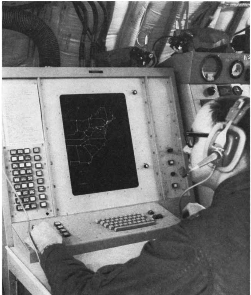
STYLIZED MAP of the eastern U.S. appears on a display console aboard an AWACS aircraft. Radar signals and identifying data are processed by computer, so that targets can be plotted against the fixed map rather than in the moving reference frame of the airplane.
