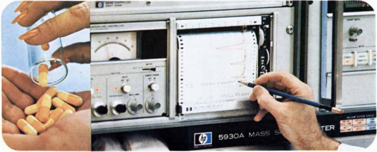
When unconscious or incoherent patients are brought into emergency, the toxicology lab can tell what drugs they may have taken, using an HP mass spectrometer.
