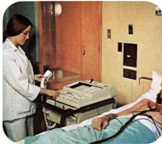
∇ The nurse is phoning an HP computer system which analyzes the patient's ECG and prints an interpretation for the physician to evaluate
