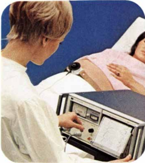
Δ During labor, this HP Fetal Monitor records the mother's uterine contractions and the baby's heart rate. These two indices help alert the doctor to conditions of fetal distress.
