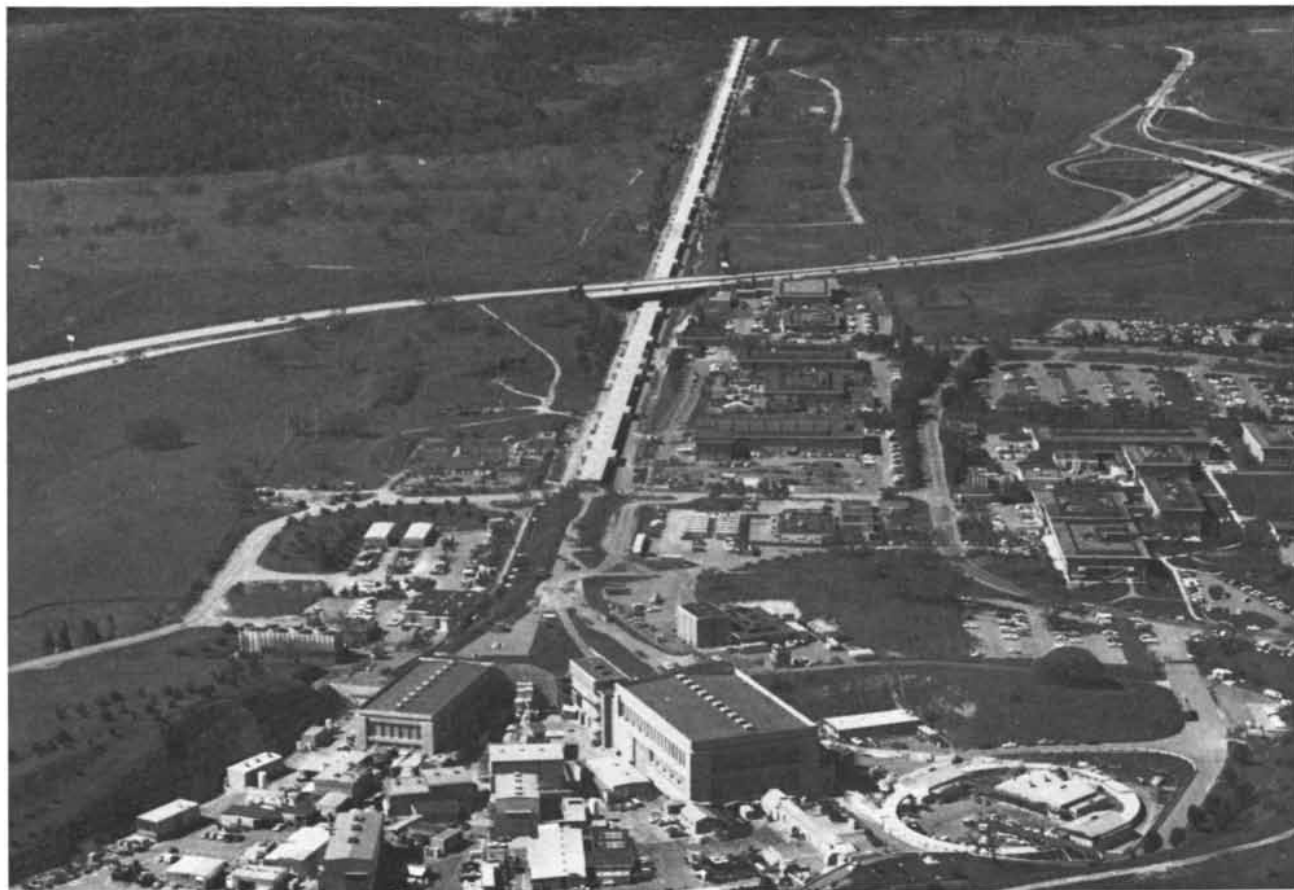
STORAGE RING at the Stanford Linear Accelerator Center is one of half a dozen such rings in the world used for experiments involving colliding beams of electrons and positrons. The ring, known as SPEAR, is visible at the lower right. It is one-seventh of a mile in
