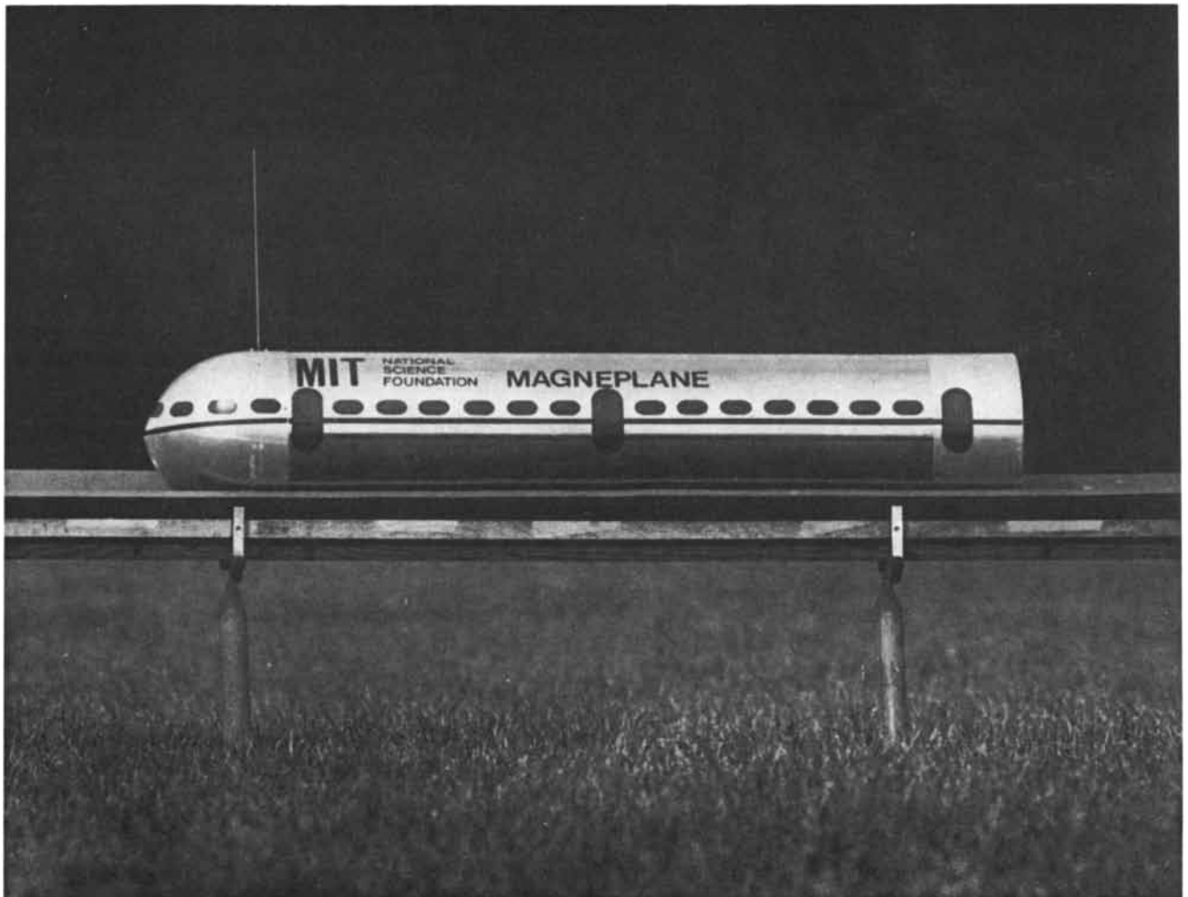
OPERATING MODEL of the magneplane is employed by the authors and their collaborators to study the motion of the vehicle
