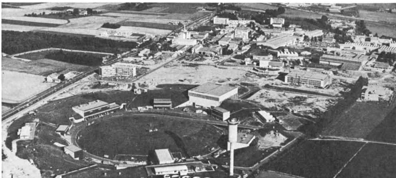
AERIAL PHOTOGRAPH of the CERN laboratory near Geneva must be examined rather closely for evidence of the two major underground proton accelerators. The large circular mound in the left foreground houses the intersecting storage rings. The somewhat smaller circular mound in the right background, partly obscured by
