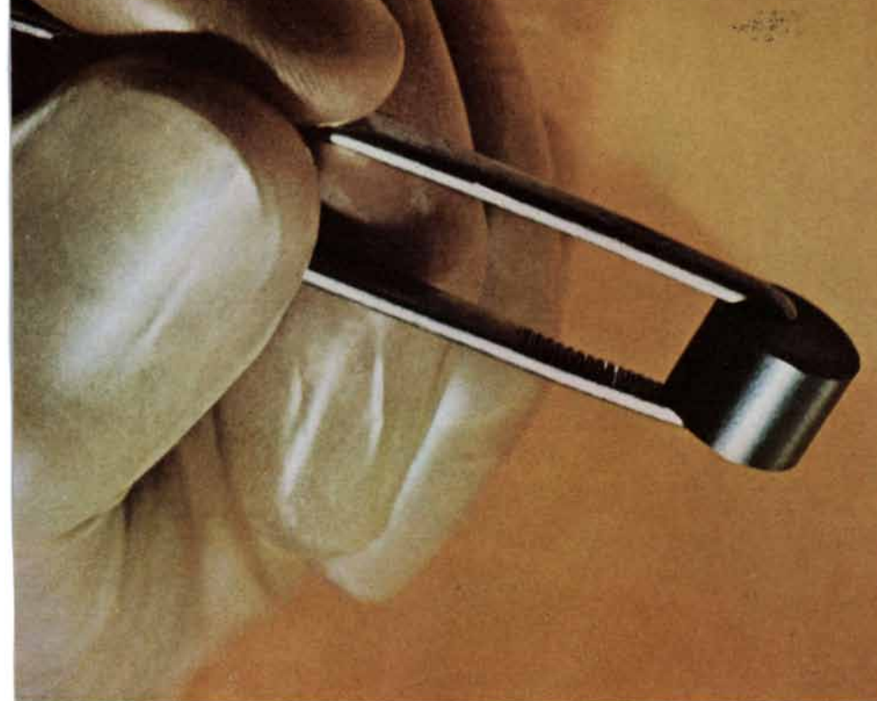
Pellets of enriched uranium (left) and fuel assemblies (right) are made by Exxon Nuclear Company. The pellets are inserted into rods, and the rods are grouped to form assemblies which make up the core or "furnace" of a nuclear reactor. An assembly, like the one shown, can generate enough electricity to run 16,000 average homes a year.
