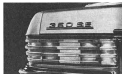
The rear light unit repels dirt, because of its ridged surface, developed in the wind tunnel.
