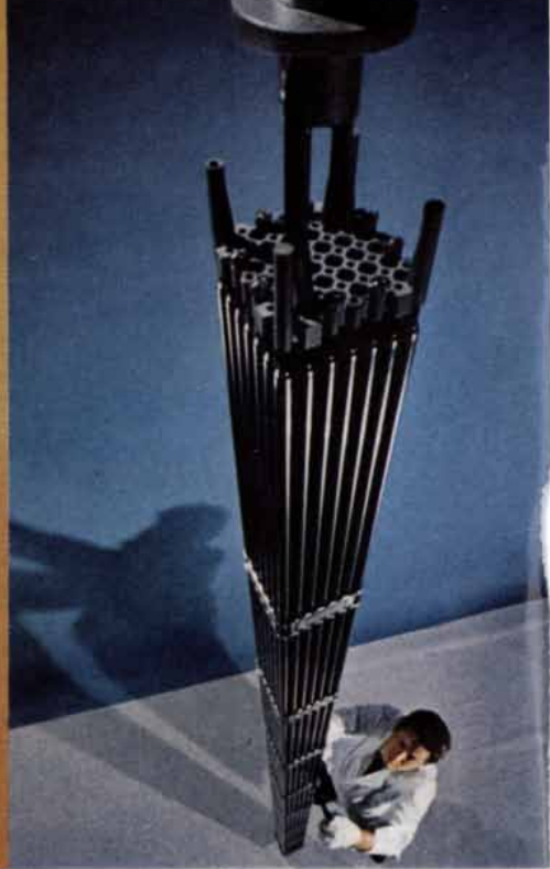
Pellets of enriched uranium (left) and fuel assemblies (right) are made by Exxon Nuclear Company. The pellets are inserted into rods, and the rods are grouped to form assemblies which make up the core or "furnace" of a nuclear reactor. An assembly, like the one shown, can generate enough electricity to run 16,000 average homes a year.
