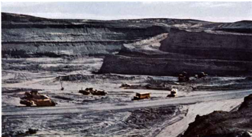
This is Exxon's uranium mine in Wyoming. When the surface mining is completed, most of the area will be filled in, contoured and planted to match the rest of the countryside. Grass, wildflowers and shrubs that Exxon planted are already growing on much of the earth that has been excavated from the mine.
