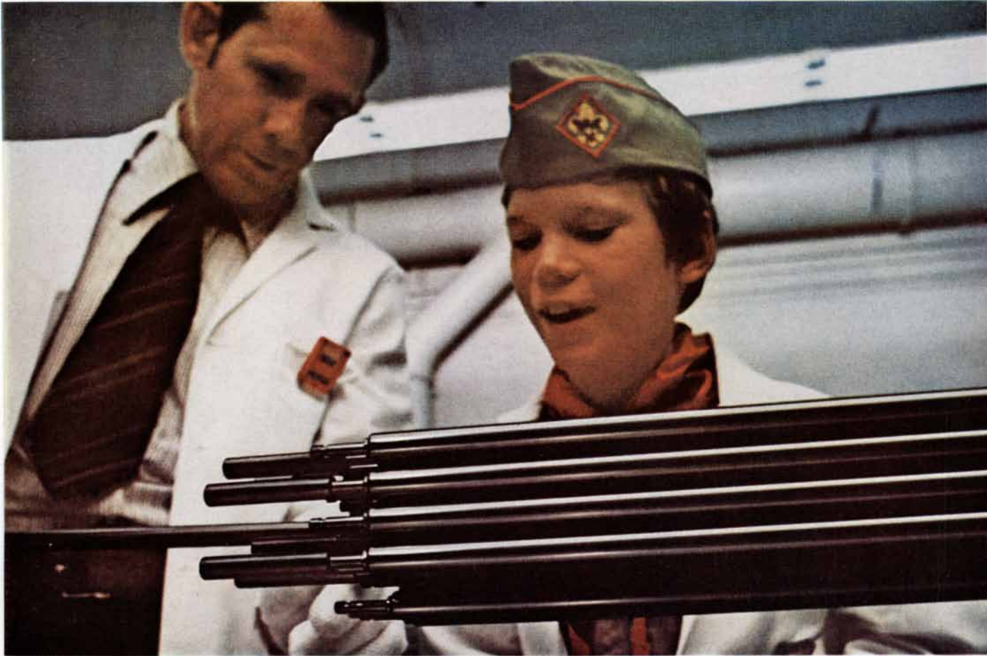
An engineer at Exxon Nuclear Company shows a young visitor how a fuel bundle is assembled. Dozens of zirconium or stainless steel tubes are filled with uranium pellets, then grouped together to form a nuclear fuel bundle. As many as 600 bundles make up the core or heat source of a reactor.
