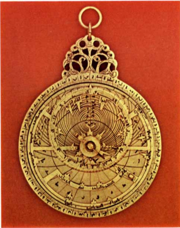
PERSIAN ASTROLABE was made in the 12th century. It is 5¼ inches across and is of fairly simple design, as are most early astrolabes. Rete is regular and star pointers are straight and unadorned.
