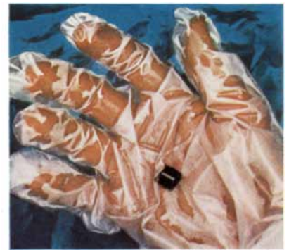
A single tiny pellet of enriched uranium can generate as much energy as 150 gallons of fuel oil. Thousands of these pellets go into a nuclear fuel bundle. A single bundle can generate enough electricity to run 4,000 average-sized homes.
