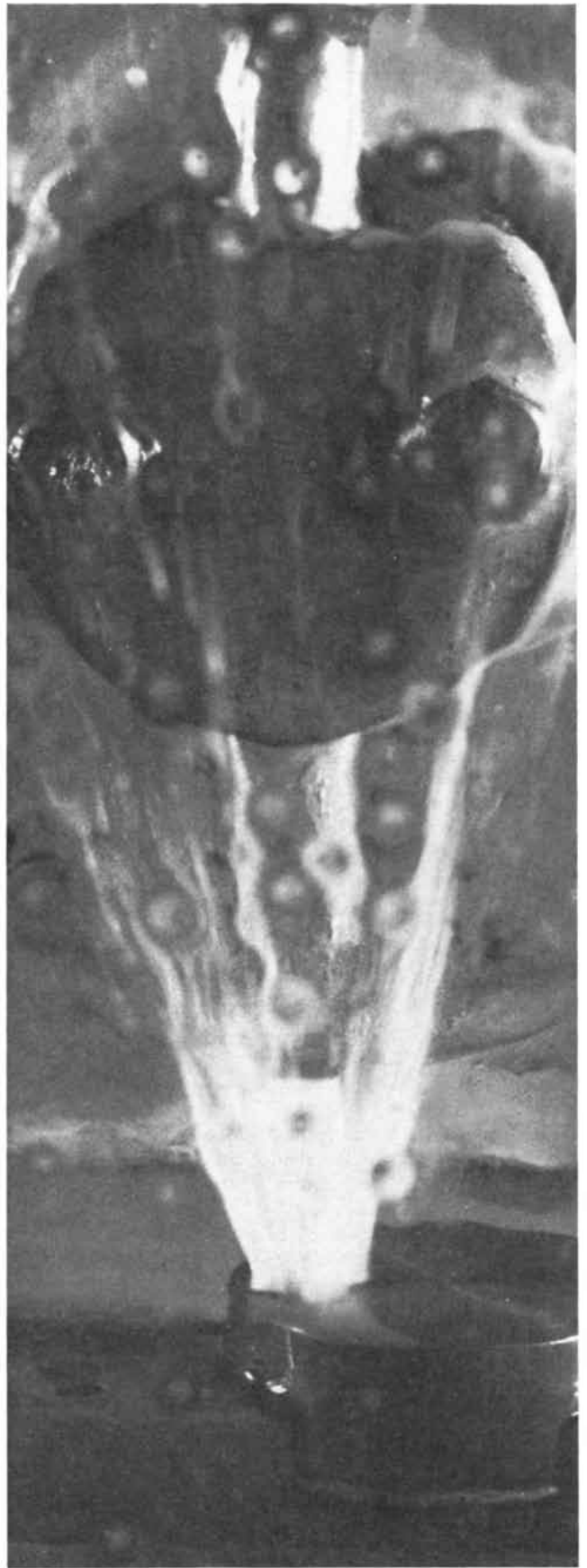
the cutting to the bottom edge of the tool. At right electrolyte fans out of the hole being cut in the workpiece. The electrolyte is pumped through center of cathode at high pressure. A gauge attached to the machine records the penetration of the cutting tool.
