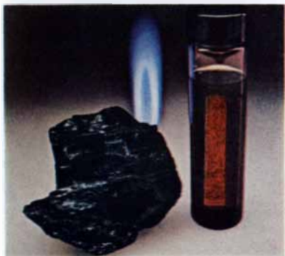
Heat and pressure applied in the right way can convert a 4-pound piece of coal into about 1 quart of synthetic crude oil or about 32 cubic feet of synthetic gas.
