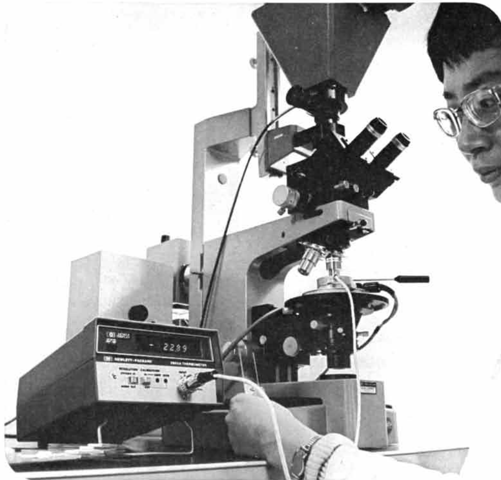
In this instance, the versatile HP 2802A thermometer measures with the repeatability of a hundredth of a degree, the transition temperature of crystal specimens.
