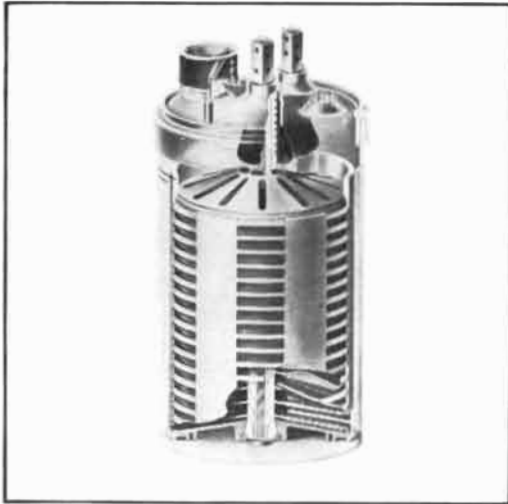
A cutaway view of the new lead-acid battery. For use in the Bell System, four types—each with a different ampere-hour capacity—will replace the 60 configurations currently in use over the same capacity range.
